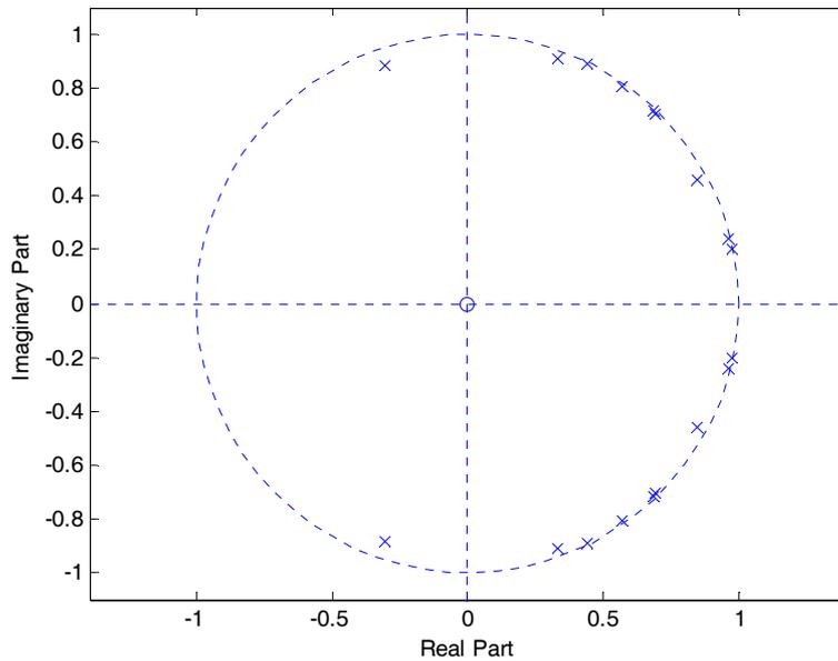
Figure 3 Poles obtained from earthquake data recorded in Y direction on 11<sup>th</sup> February, 2006
