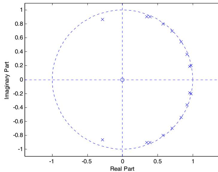
Figure 5 Poles obtained from earthquake data recorded in Y direction on 12<sup>th</sup> August, 2006
