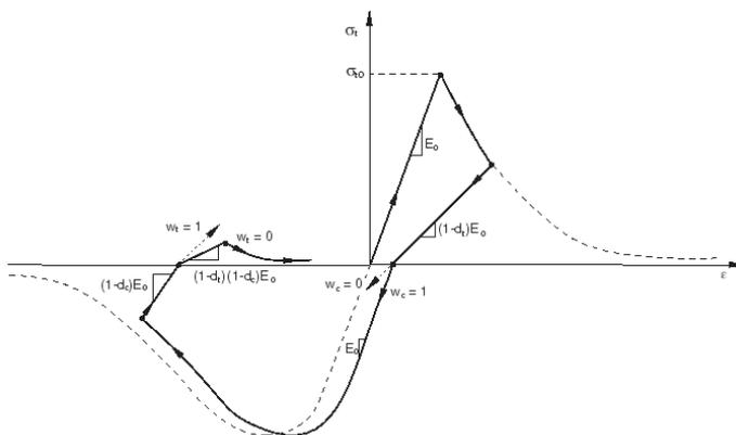
Figure 1 Concrete tension-compression stiffness restoration curve
