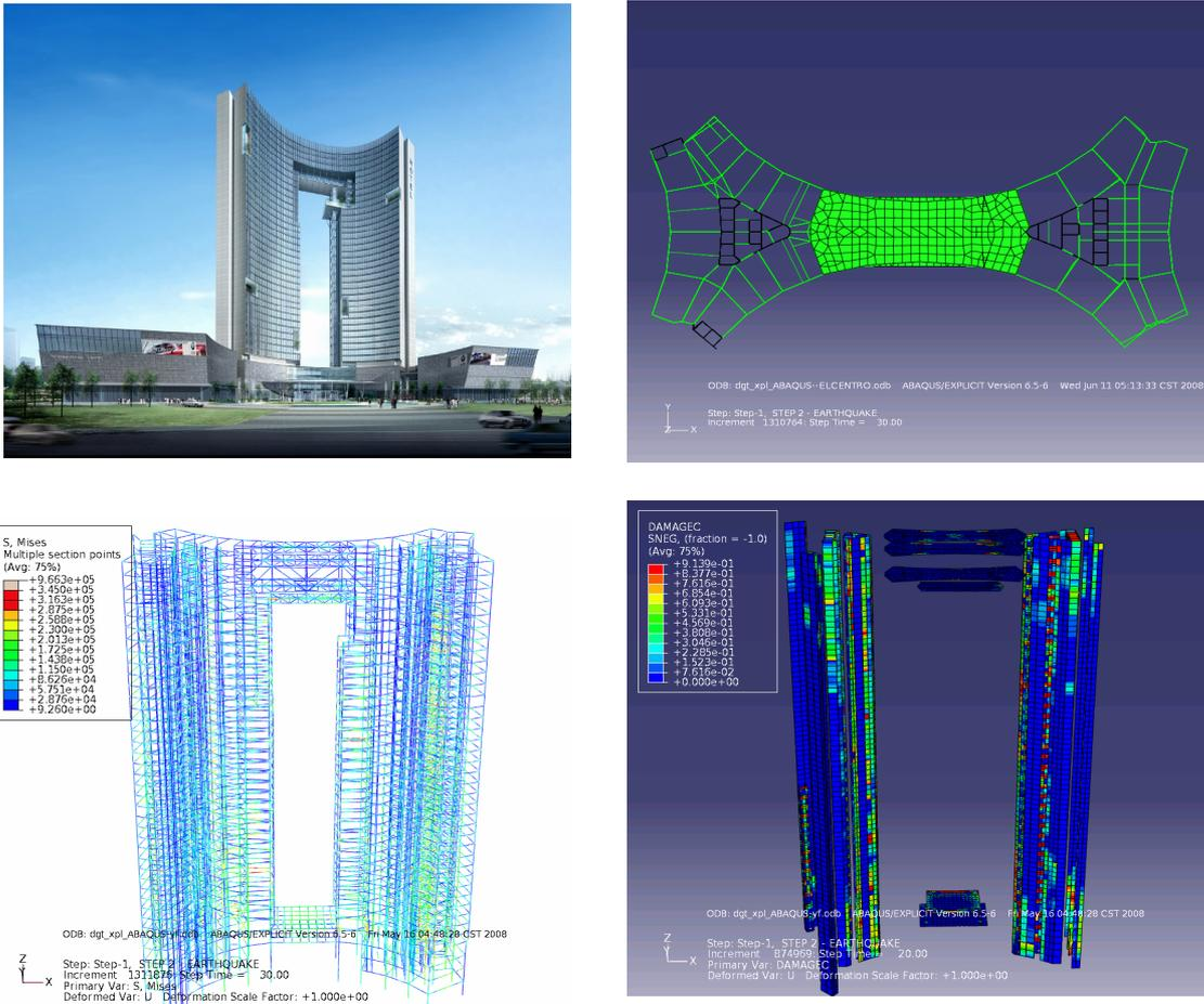
Figure 4 Three-dimensional effect, the floor plan, overall Mises stress and shear wall compression damage
