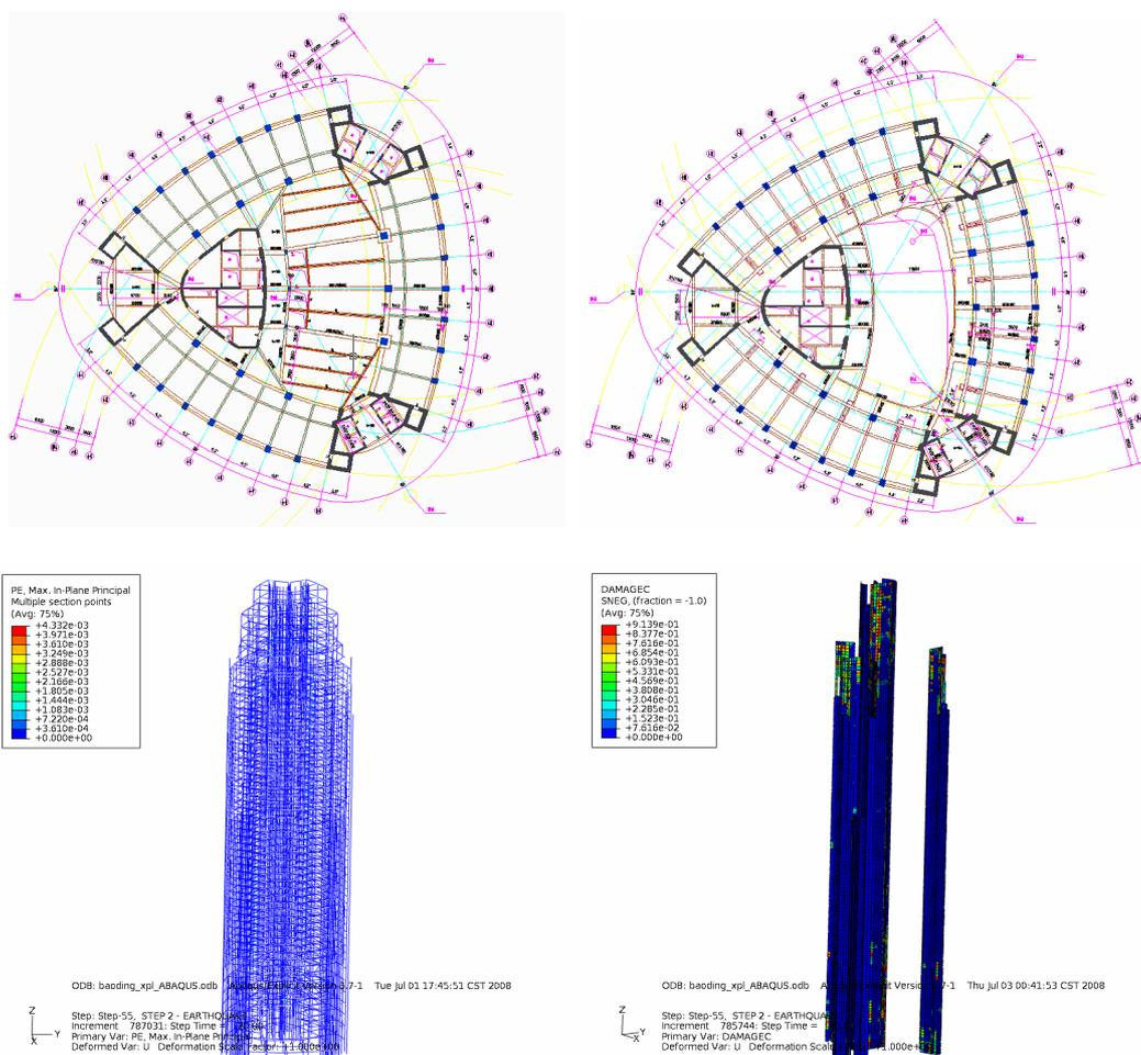
Figure 5 The 28<sup>th</sup> transfer layer, the standard floor plan, the plastic strain and shear wall compression damage
