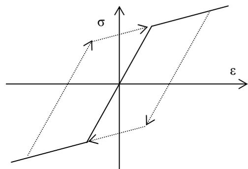
Figure 2 Steel tension-compression hysteretic curve
