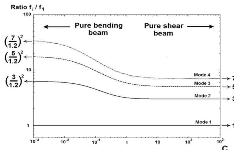
Figure 6 Distribution of the eigenfrequencies of a Timoshenko beam according to the dimensionless parameter  $C$
