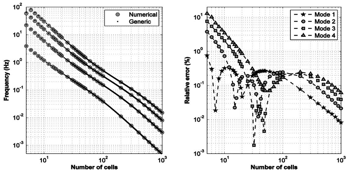
Figure 5 Comparison between numerical calculations and generic model according to the number of cells for the four first modes
