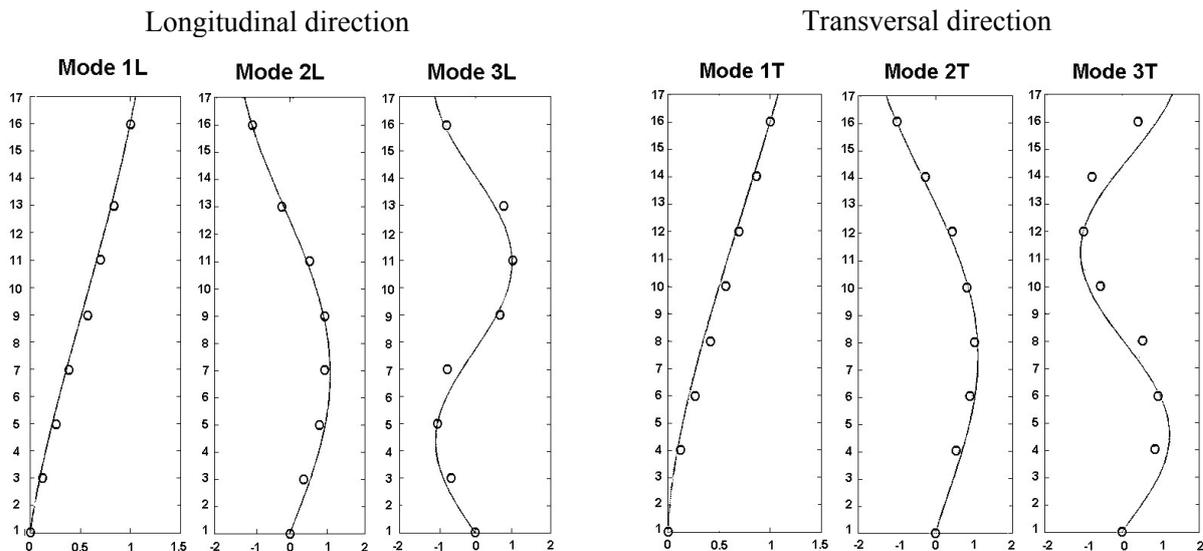
Figure 7 Comparison between the theoretical (line) and experimental (points) modal shapes
