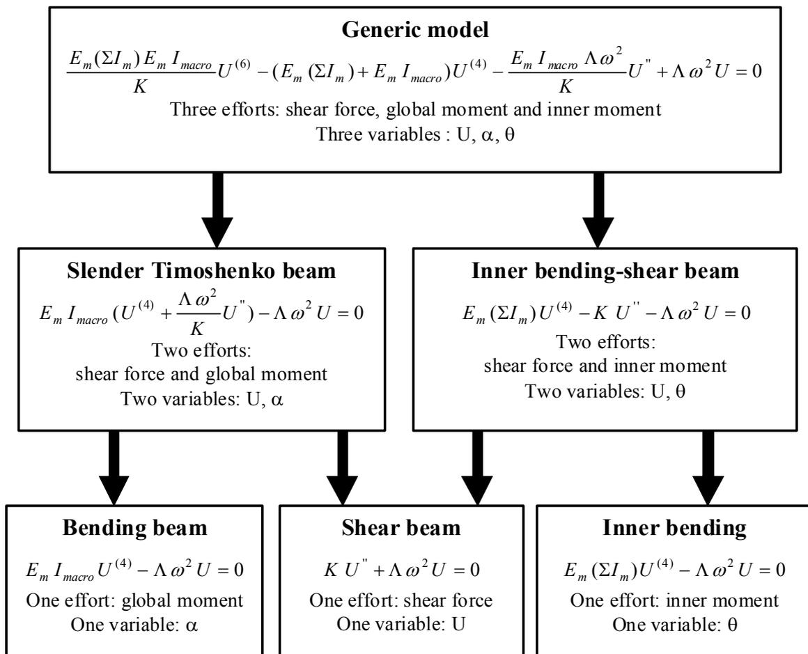
Figure 3 Beam models with the driving efforts and variables
