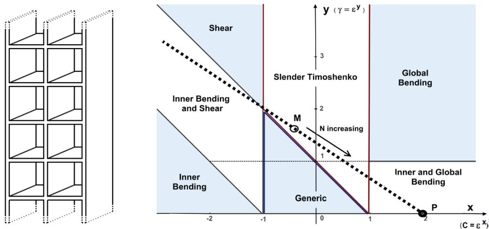
Figure 4 Left: double frame structure, right: domains of validity of the beam models
