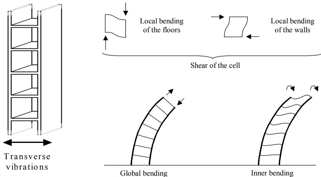
Figure 2 Left: class of studied structure, right: mechanisms governing the transverse vibrations
