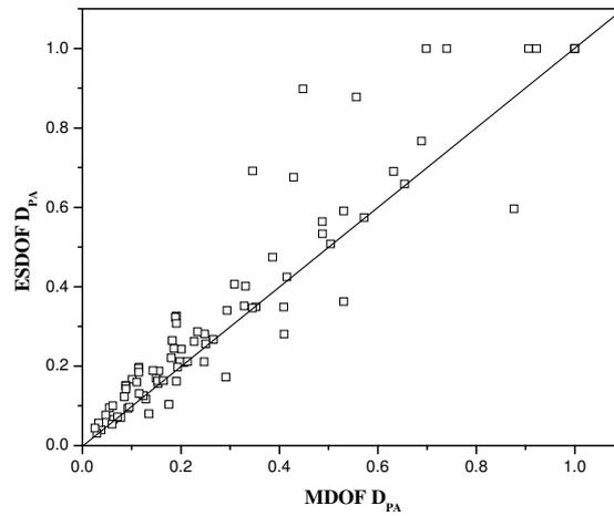
Figure 2 Scatterplot comparing D<sub>PA</sub> values of MDOF and ESDOF system for the 3-story frame
