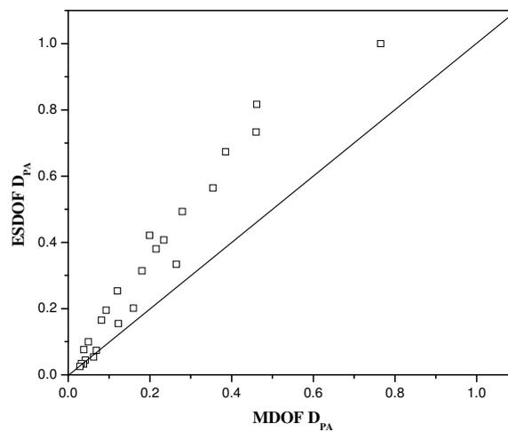
Figure 4 Scatterplot comparing D<sub>PA</sub> values of MDOF and ESDOF system for the 20-story frame
