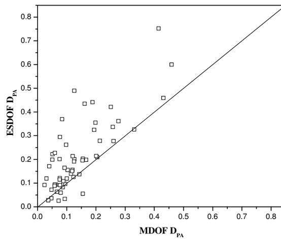
Figure 3 Scatterplot comparing D<sub>PA</sub> values of MDOF and ESDOF system for the 9-story frame
