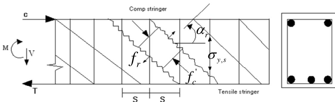
Figure 2 Beam with vertical stirrup and concrete stress.
