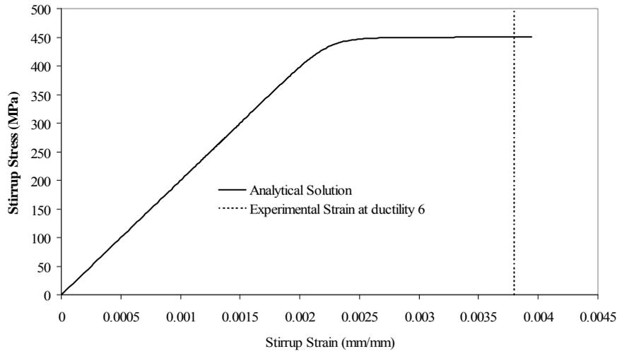
Figure 5 Transverse reinforcement stress-strain behavior
