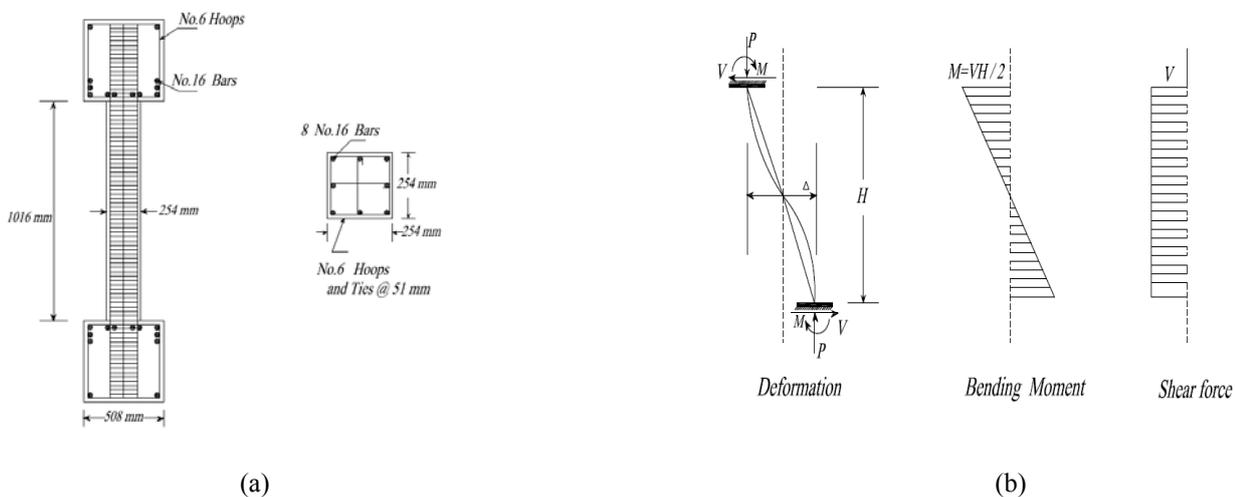
Figure 3 (a) Column details and (b) Loading pattern.
