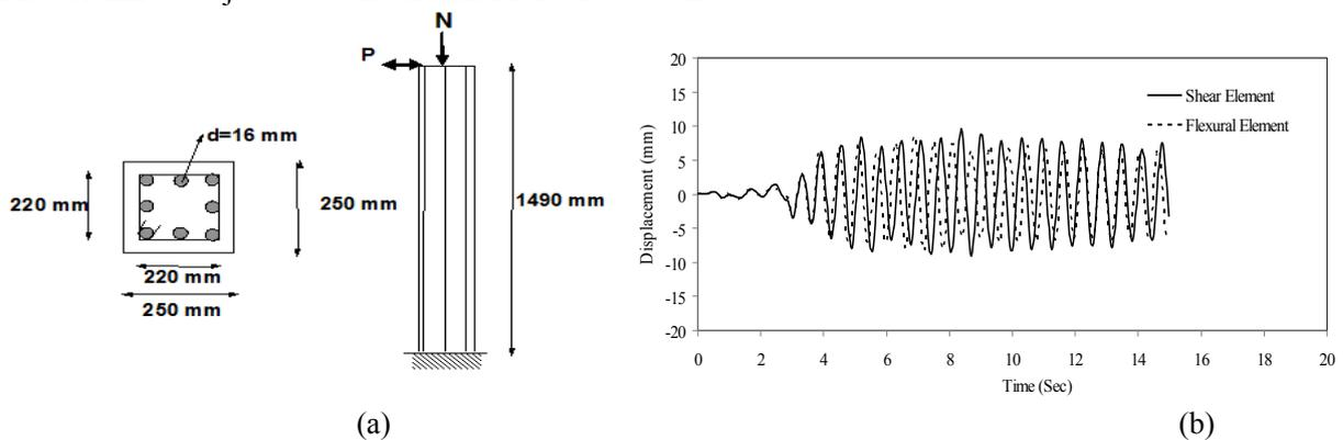
Figure 6 (a) Column details (b) Earthquake response of Bousias column with Erzincan earthquake record
