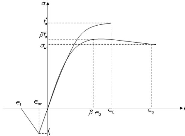
Figure 1 Stress-Strain curve with softening (1990)
