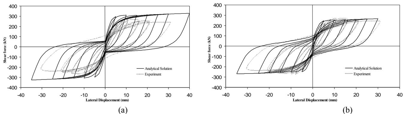
Figure 4 Cyclic shear force displacement hysteresis comparison with experiment (a) flexural element (b) shear element
