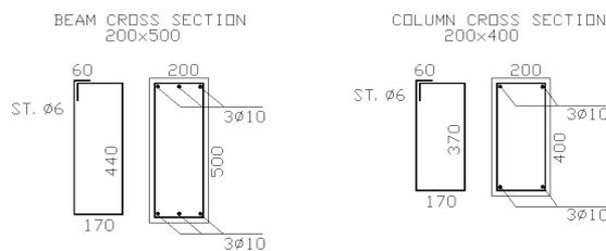
Figure 1. Details of beams (right) and columns (left) cross section.
