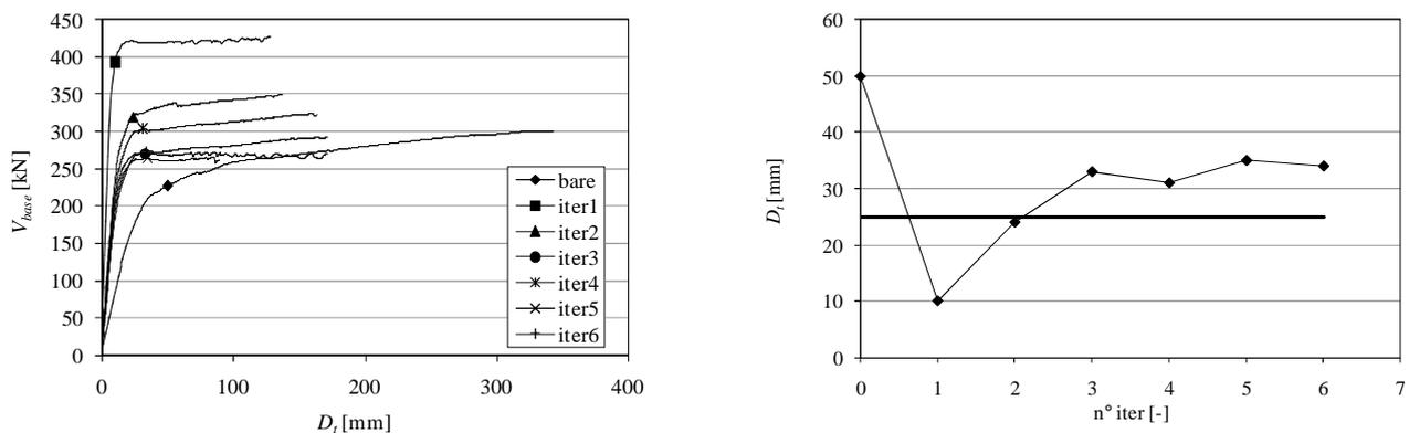
Figure 3. (a) BRB effect on capacity curves, (b) Performance top displacement of the braced frame at each step (iter=0 is the original frame).
