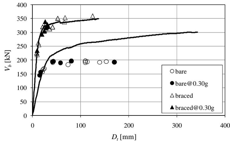
Figure 4. Capacity curves vs. incremental nonlinear dynamic analyses of bare and braced frame.
