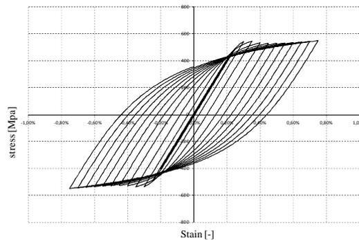
Figure 3. Cyclic model of the reinforcing steel.
