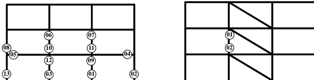
Figure 5. Damage distributions of existing and retrofitted frame.
