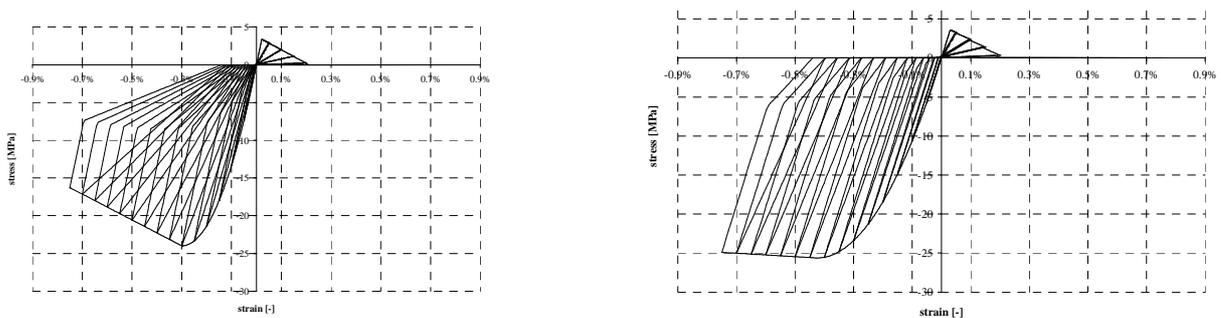
Figure 2. Cyclic model of unconfined and confined concrete.
