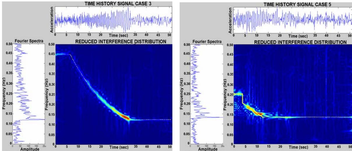
**Figure 2-1 Reduced Interference Distribution of Typical Structures (Left: Signal # 3 Slowing Stiffness Decrease as flexural damage, Right: Signal #5, Sudden Stiffness Decrease as shear damage)**
