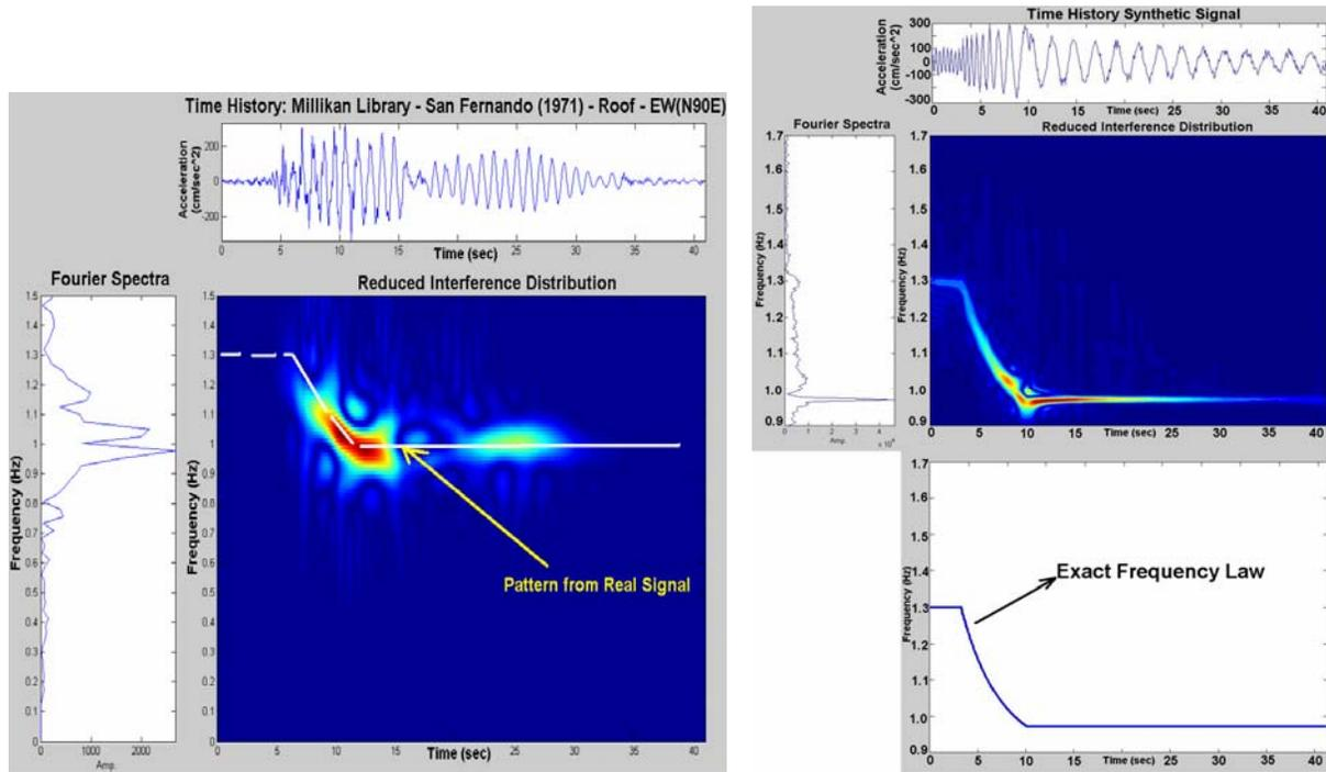
Figure 3-2 Left side: TFRs of San Fernando Earthquake (1971) recorded in Millikan Library (EW-Roof Component), Right side: TFR of Synthetic Signal and its theoretical frequency law to this record
