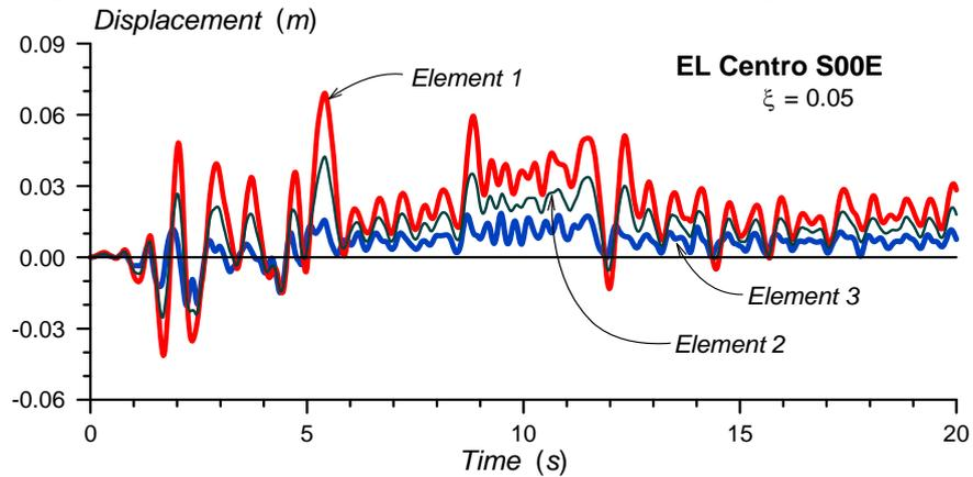
Figure 6b. Restrained system – displacement time history
