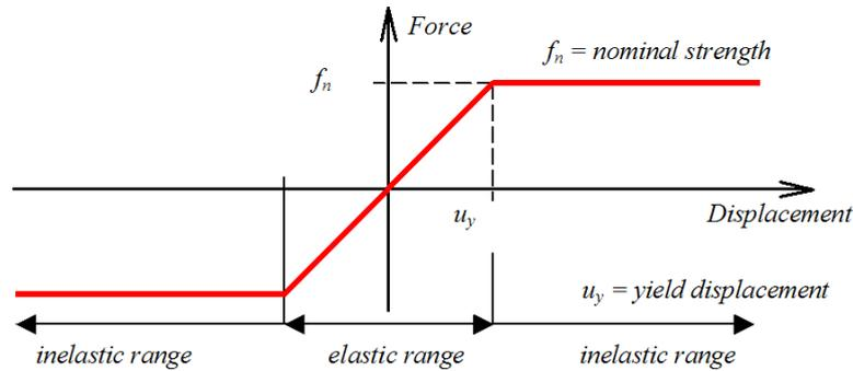
Figure 1. Elasto-plastic force displacement relationship of resisting elements
