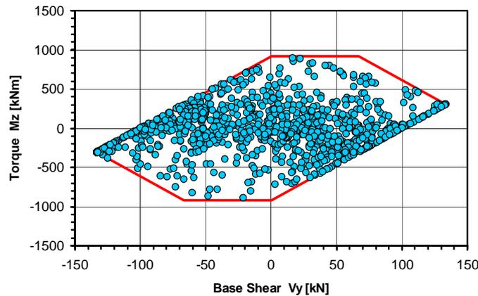
Figure 5a. Unrestrained system – base shear and torque response histories
