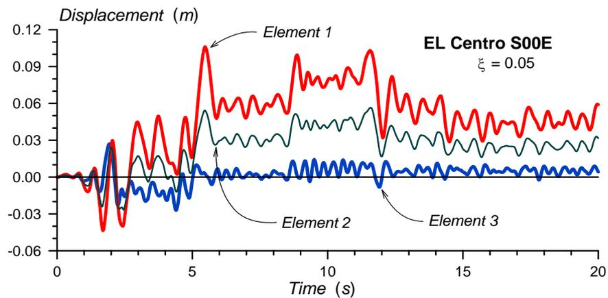
Figure 5b. Unrestrained system – displacement time history
