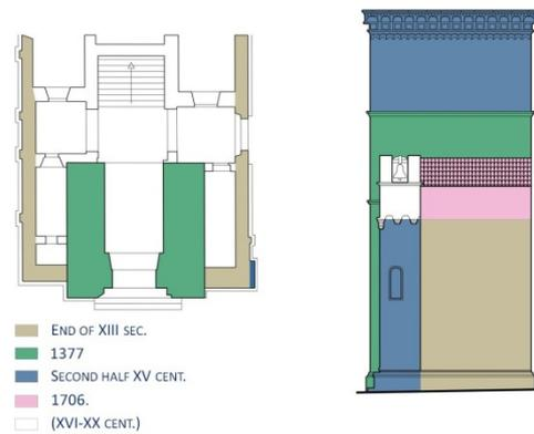
Figure 1 Bell tower construction phases
