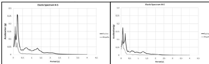
Figure 8 Majella and Fucino earthquake spectra obtained from the accelerograms deconvoluted to the base of the soil domain
