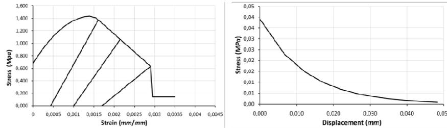
Figure 5 (a) inelastic compressive behavior, (b) tensile behavior
