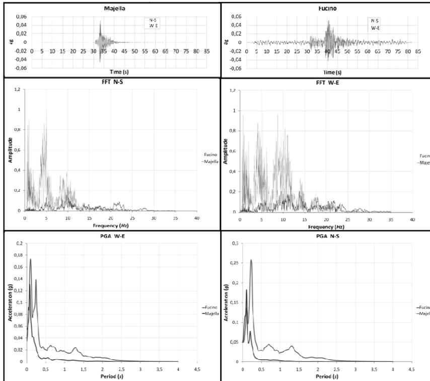
Figure 7 Majella and Fucino earthquakes at the base of the bell tower
