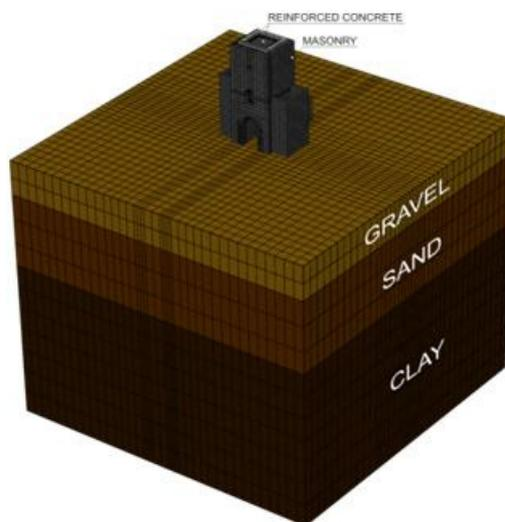
Figure 4 Soil domain stratigraphy and FE model
