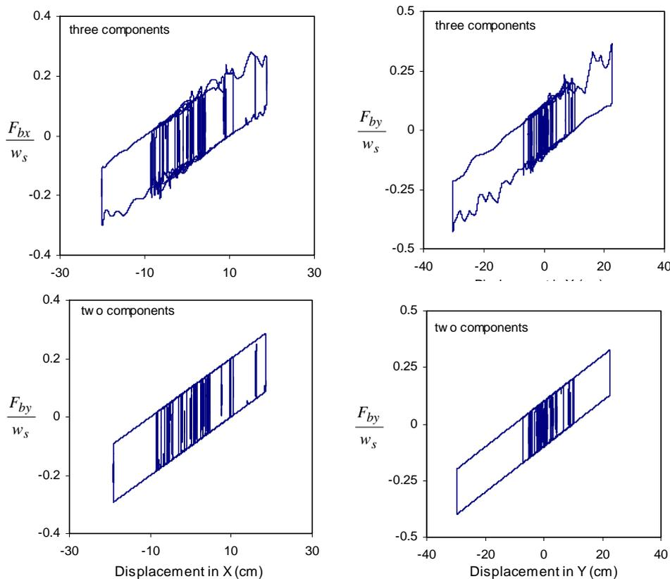
Figure 3 Hysteresis loops of bearing in X and Y directions under two and three components of Tabas earthquake excitation ( $T_i = 2s$ ,  $T_s = 0.1s$ ,  $f_{max} = 0.1$ )
