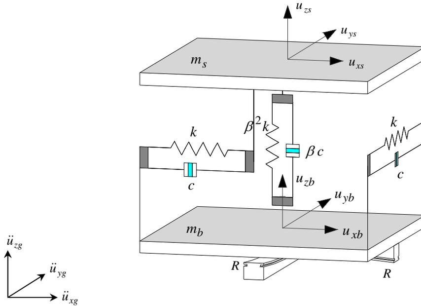
Figure 2 Idealized three-dimensional single-story structure resting on XY-FP bearing
