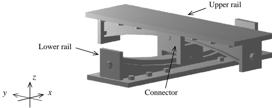
Figure 1 3D drawing of XY-FP bearing (Roussis, 2004)
