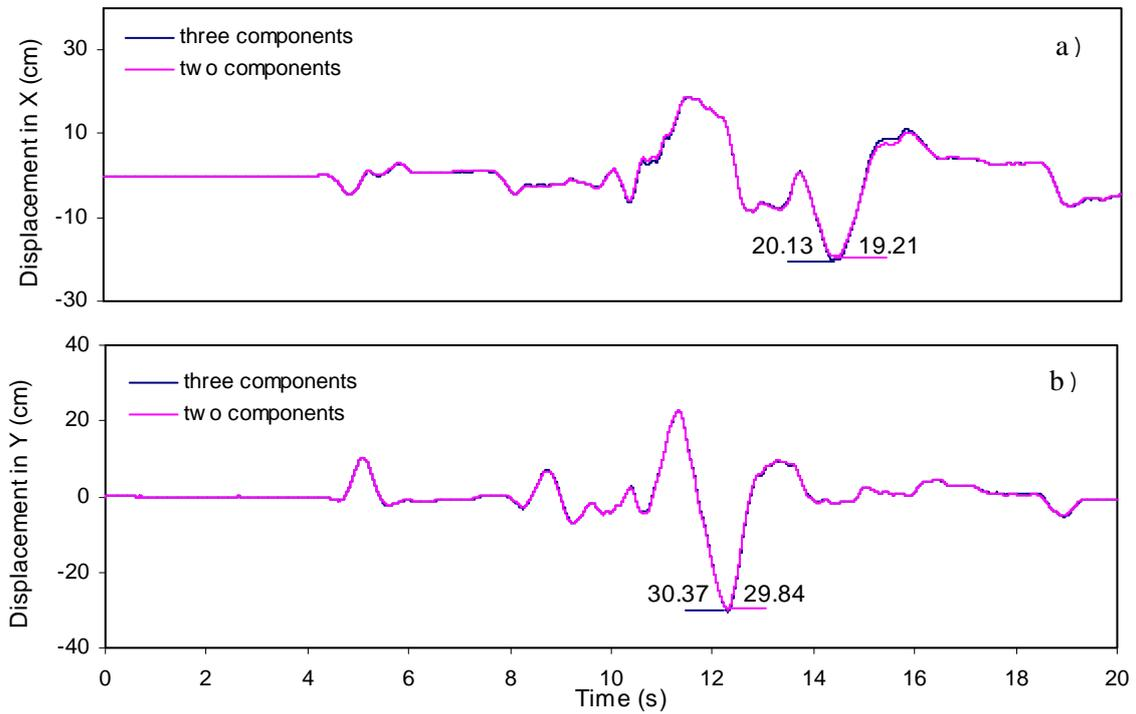
Figure 4 Time variation of bearing displacement in (a) X and (b) Y directions under Tabas earthquake excitation ( $T_i = 2s, T_s = 0.1s, f_{max} = 0.1$ )
