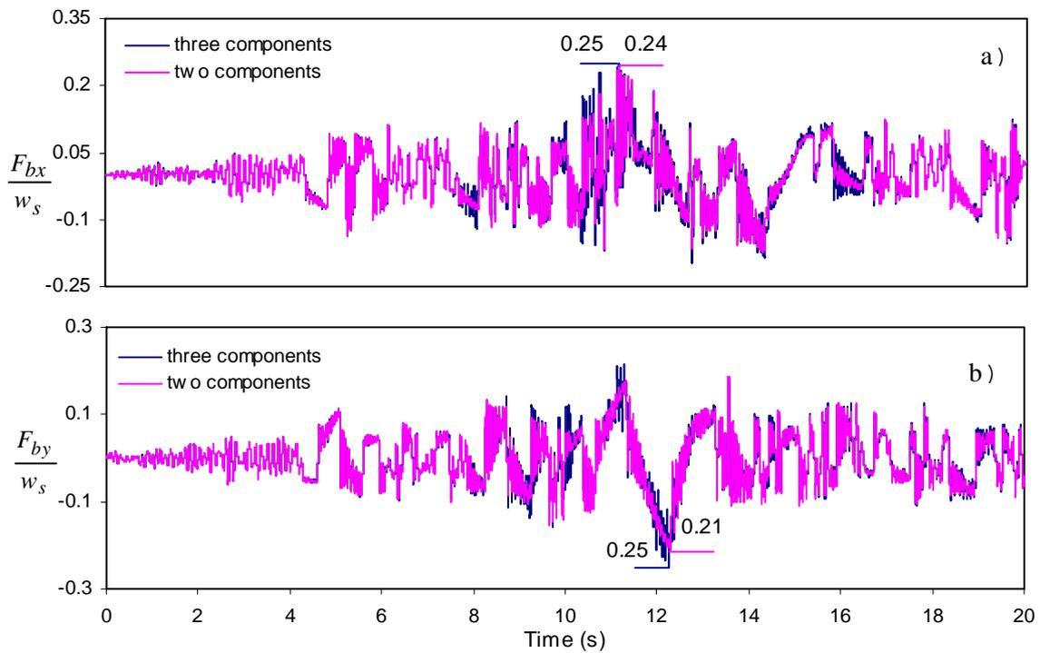
Figure 5 Time variation of base shear in (a) X and (b) Y directions under Tabas earthquake excitation ( $T_i = 2s, T_s = 0.1s, f_{max} = 0.1$ )
