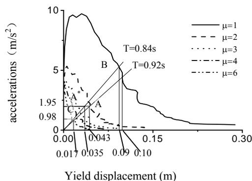
Fig.3 Estimating displacement response of the pier by inelastic seismic demand spectrum with  $A_y - D_y$  format (case 1)
