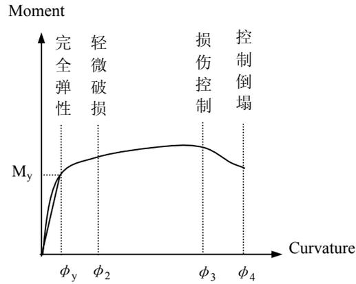
Fig.2 Bending Moment - curvature relationship of cross section at the bottom of the pier
