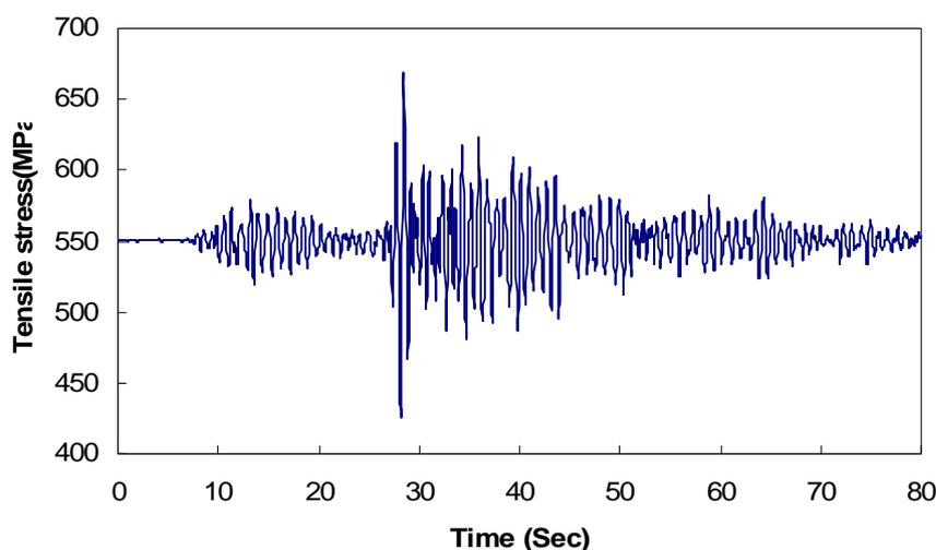
Figure 6 Time History of Tensile Stress in Cable 14
