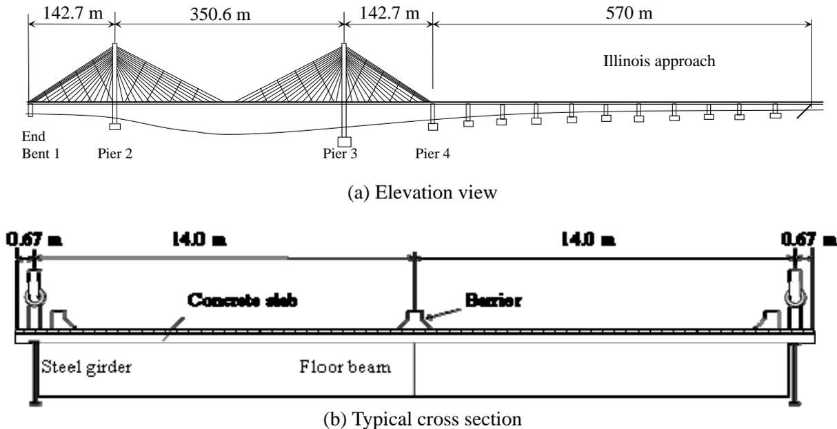
Figure 1 Schematic view of the Bill Emerson Memorial Cable-stayed Bridge
