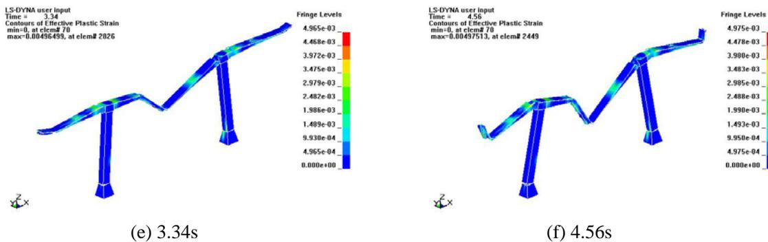
Figure 5 The simulation of the damaged mechanism and collapse mode of the bridge during strong earthquake motion
