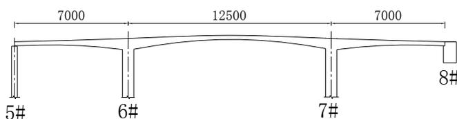
Figure 1 The elevation drawing of the bridge(cm)
