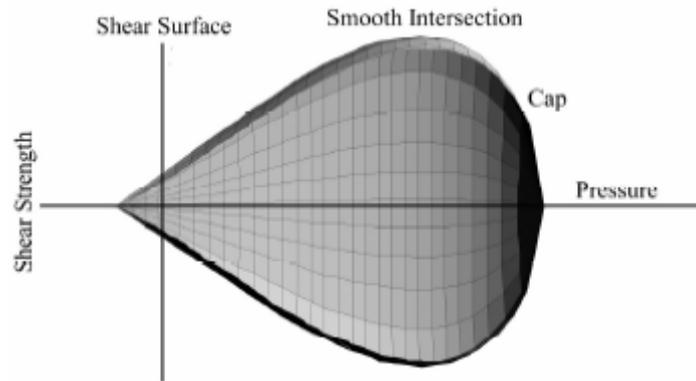
Figure 3 General shape of the concrete model yield surface in two-dimensions
