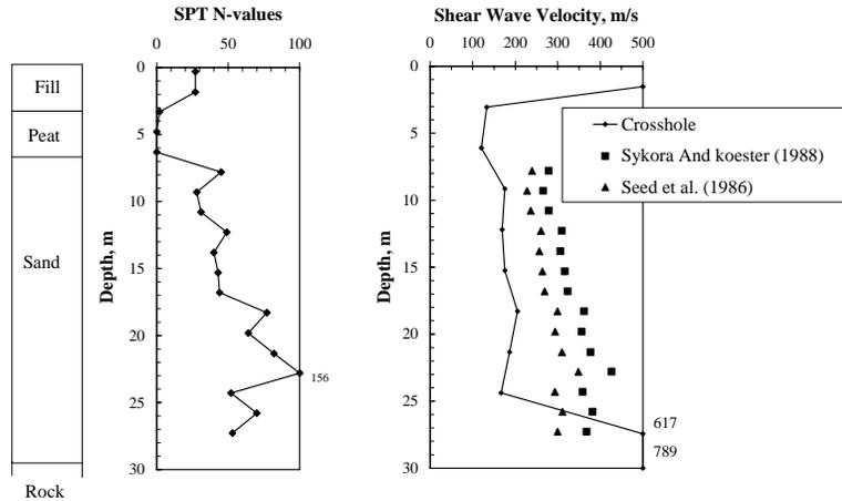
Figure 10 Comparisons of measured and estimated shear wave velocities.
