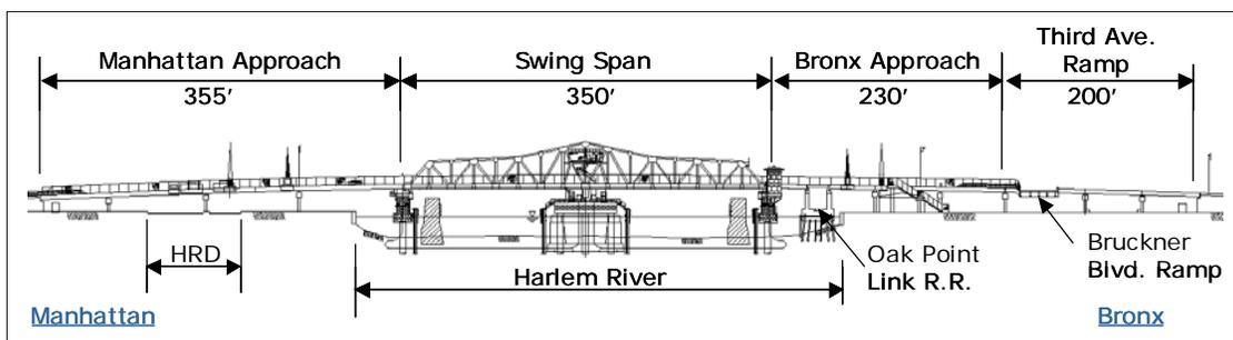
Fig. 4 General Elevation of New Third Avenue Bridge
