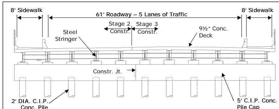
Fig. 8 Typical Section Through the Manhattan Approach
