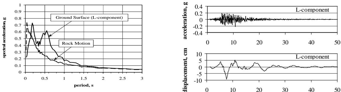
Figure 11 Generated spectra and time-history records used in the SSI analysis.
