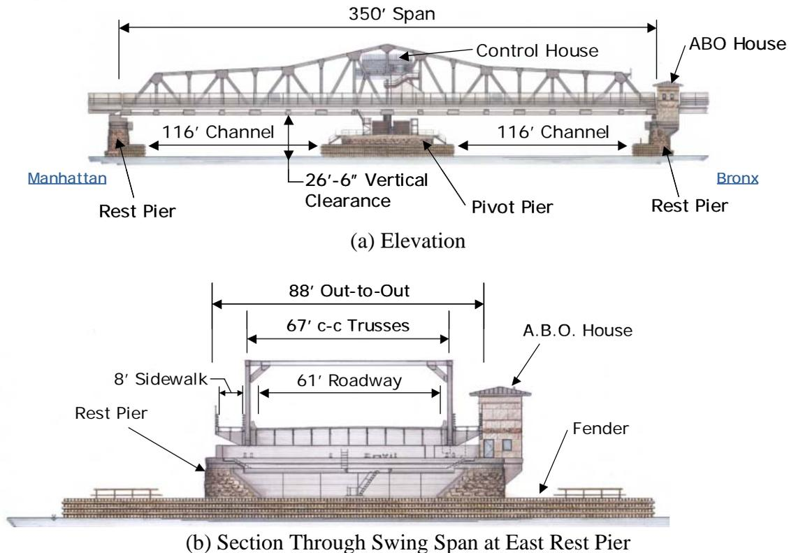
Fig. 5 Rendering of New Third Avenue Bridge Swing Span
