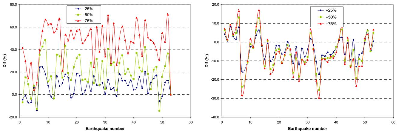
Figure 4.4 Transversal displacements in the node three. Modification of the extreme pier length
