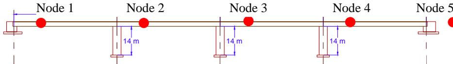
Figure 4.1 Nodes where seismic responses were evaluated
