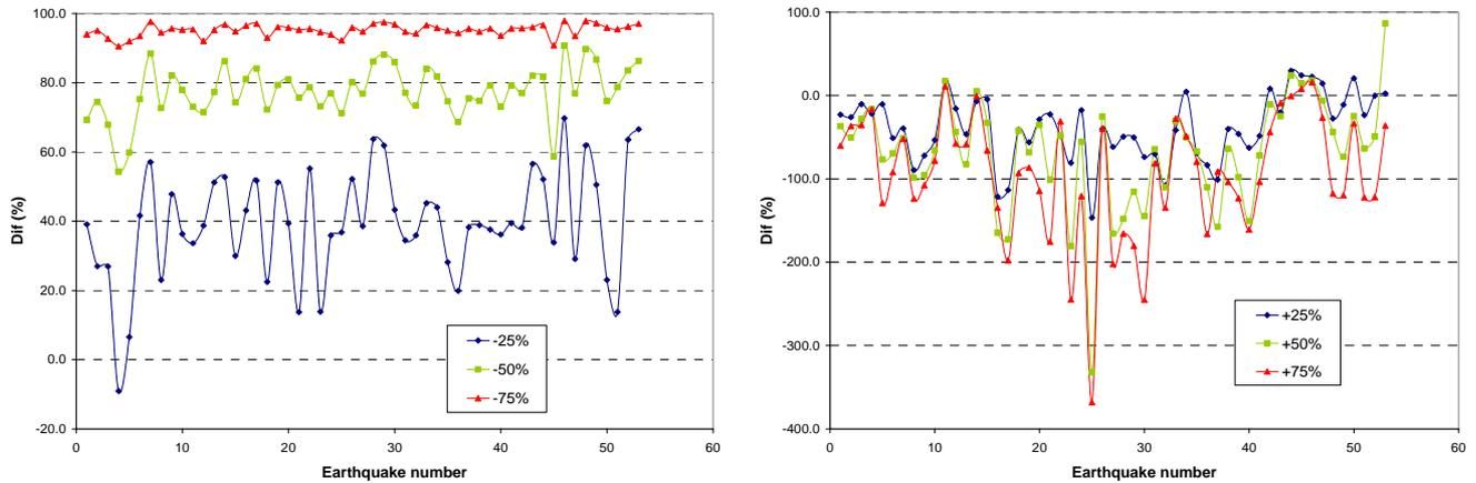
Figure 4.3 Longitudinal displacements in the node three. Modification of the central pier length
