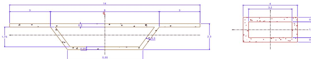
Figure 2.2 Cross section of girder (left) and piers (right)
