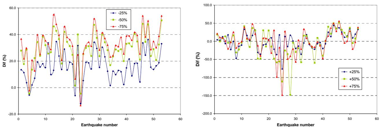
Figure 4.5 Longitudinal displacements in the node three. Modification of the extreme pier length
