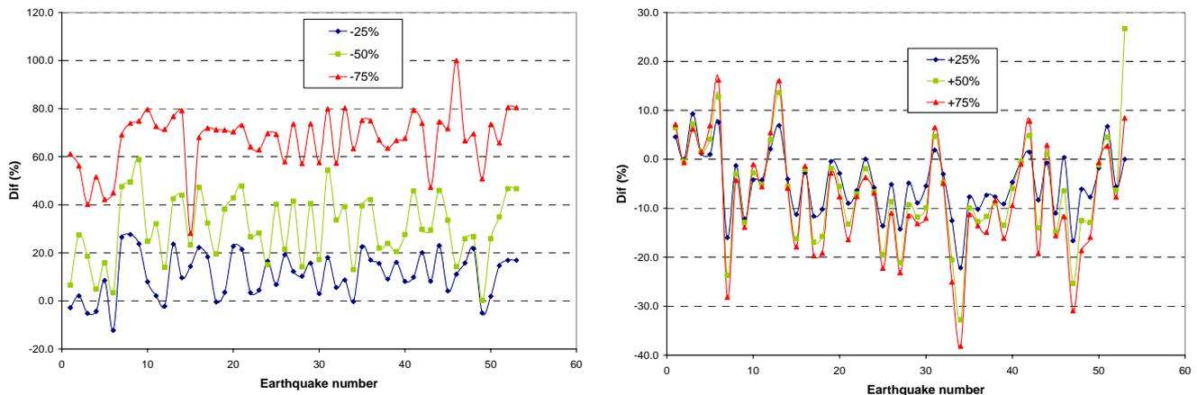
Figure 4.2 Transversal displacements in the node three. Modification of the central pier length
