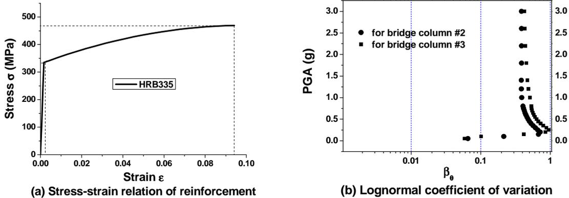
Figure 4 Reinforcement model and the variation of  $\theta_{max}$  in IDA
