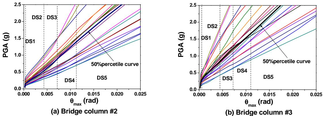
Figure 5 IDA curve in bridge columns for 20 earthquakes
