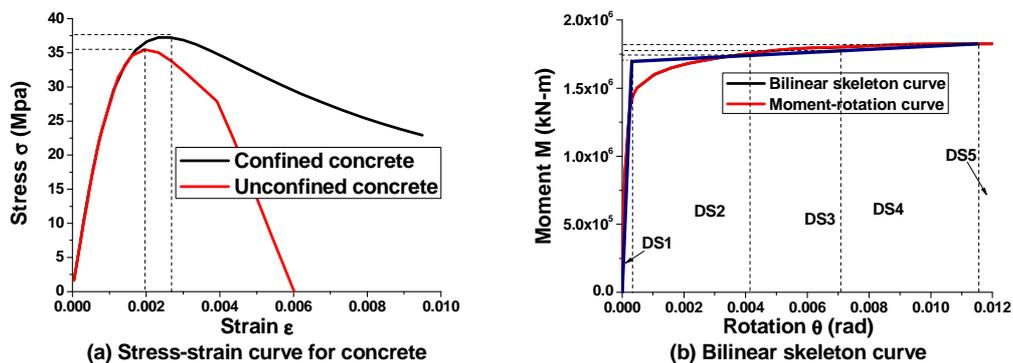
Figure 3 Concrete model and skeleton curve for Takeda hysteretic model
