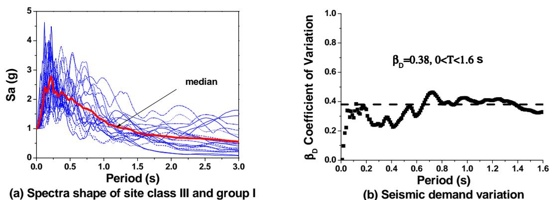
Figure 1 Ground motion records normalized to dynamic amplification factor
