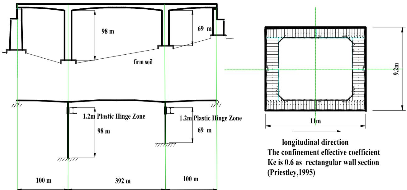
Figure 2 Bridge model and critical sections
