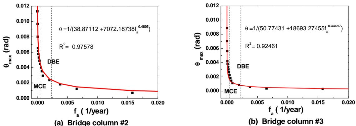
Figure 6 Fitted rotation hazard curves for 50% percentile IDA curve
