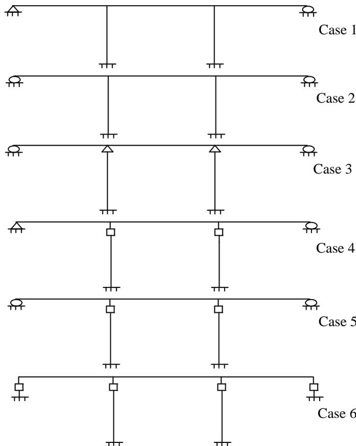
Figure 4 Different bearing arrangements considered for the study
