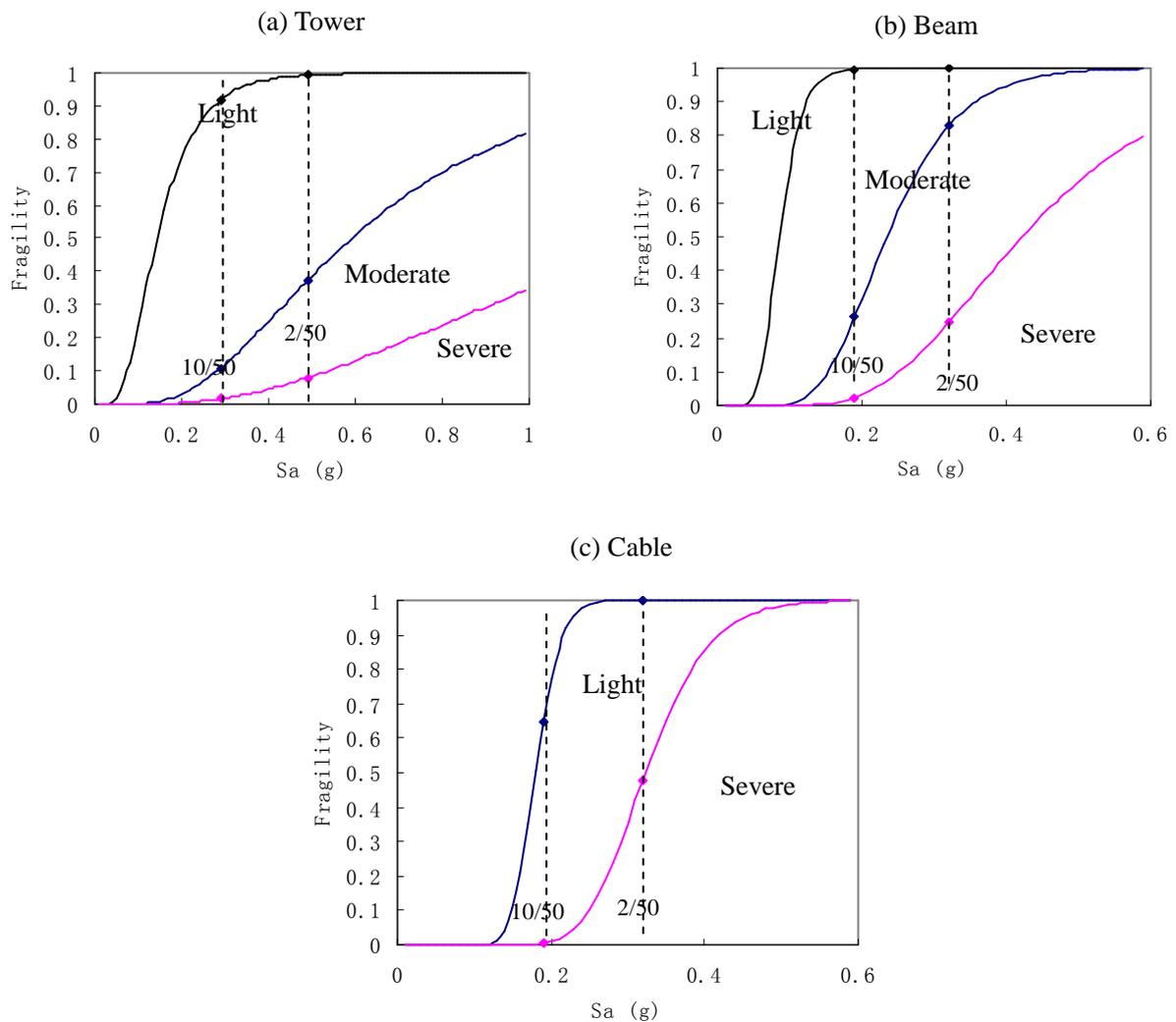
Fig 6. Fragility curves of tower, beam and cable
