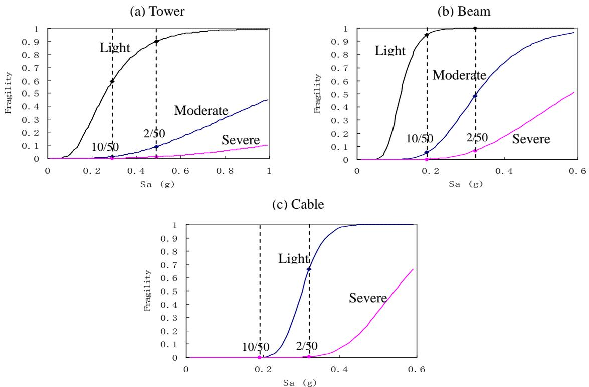
Figure 5. Fragility curves of tower, beam and cable
