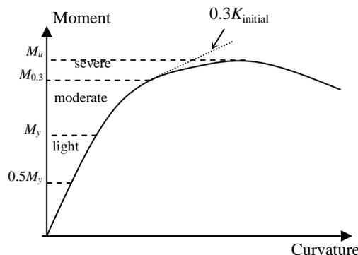
Figure 4 Damage states defined corresponding to internal moment
