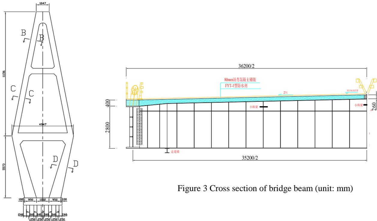
Figure 3 Cross section of bridge beam (unit: mm)
