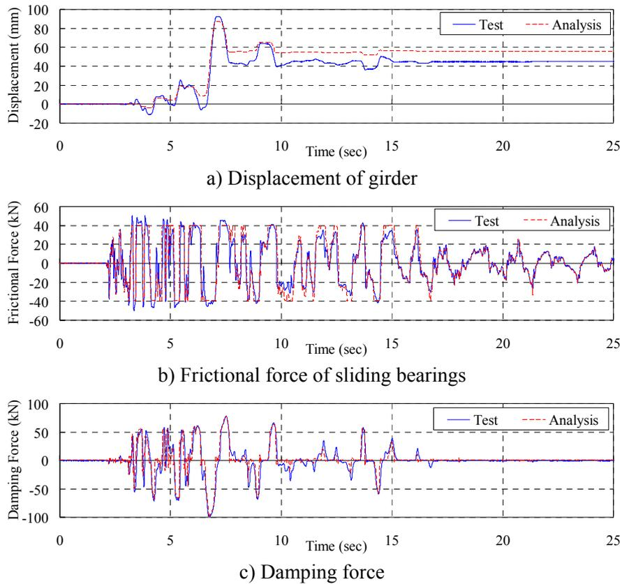
Figure 8 Analytical simulation in Case3 (damper type 1, input amplitude 100%)
