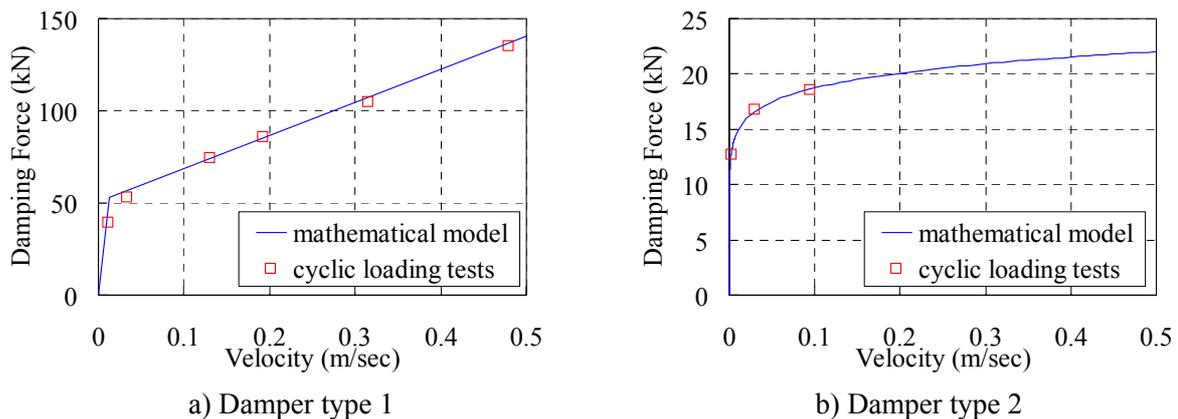
Figure 1 Damping force dependency on loading velocity
