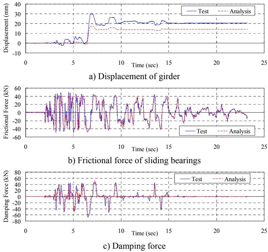
Figure 6 Analytical simulation in Case1 (damper type 1, input amplitude 70%)
