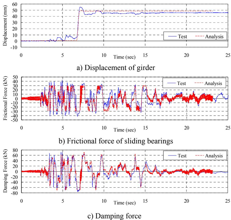
Figure 11 Analytical simulation in Case6 (damper type 2, input amplitude 100%)
