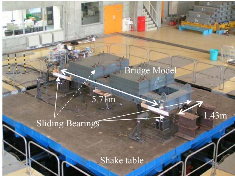
Figure 2 Setup of bridge model
