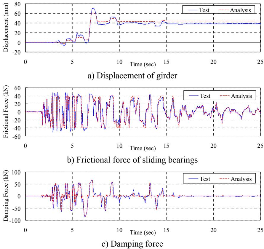
Figure 7 Analytical simulation in Case2 (damper type 1, input amplitude 90%)
