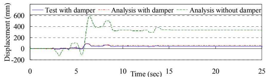
Figure 12 Damping effect for displacement
