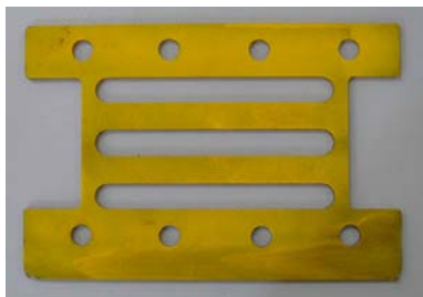
Fig 4(a) Strip metallic damper Fig 4(b) Hysteretic curves of strip metallic damper
