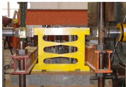
Fig 7 Test setup of prototype damper
