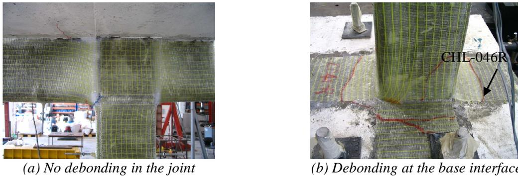
Figure 6 Close-up of observed damage of repaired frame after 0.46g test
