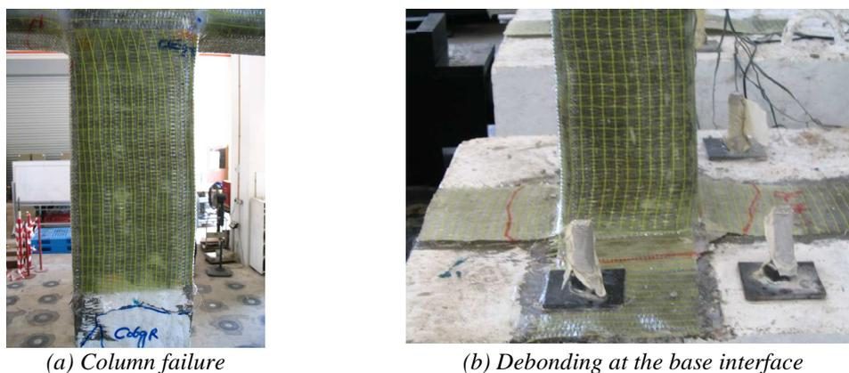
Figure 7 Close-up of observed damage of repaired frames after CHL-069R
