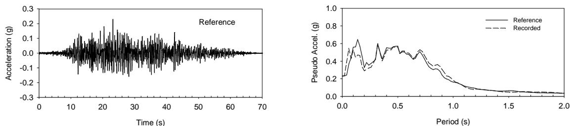
Figure 2 Accelerogram and response spectra of the simulated ground motion
