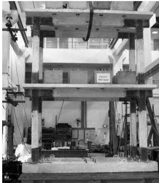
Figure 4 FRP repaired frame
