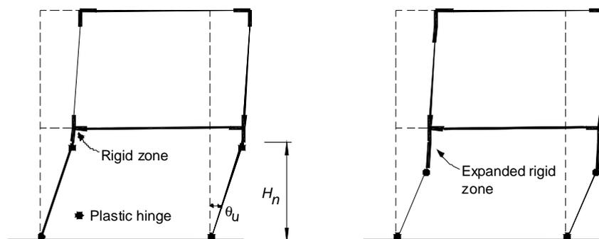
Figure 9 Schematic of final failure modes of test frame
