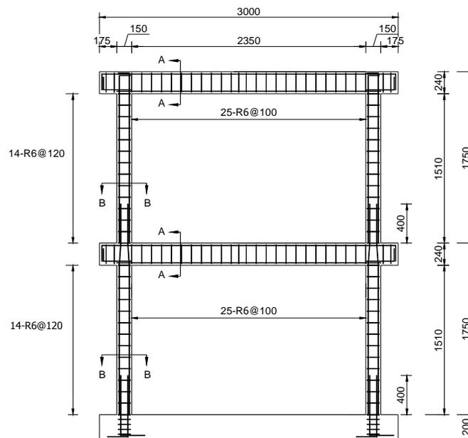
Figure 1 Geometry of test frame
