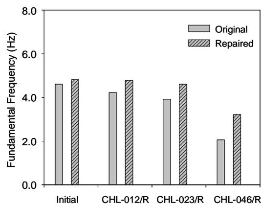
Figure 5 Fundamental frequencies of test frames (original and repaired)
