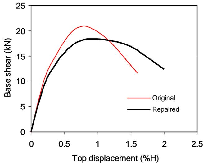
Figure 8 Base shear vs. top displacement envelopes of test frame
