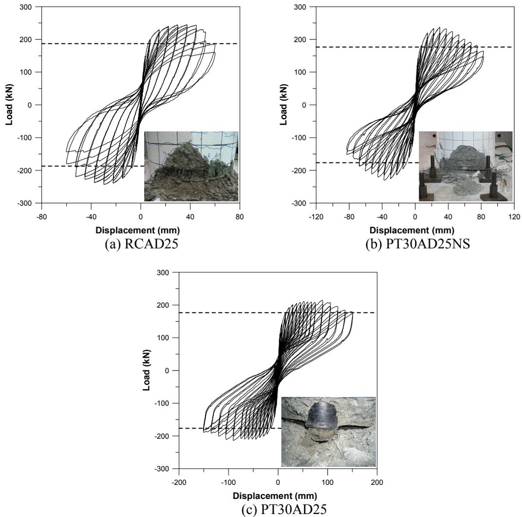
Figure 4 Lateral load-displacement relationship for specimens
