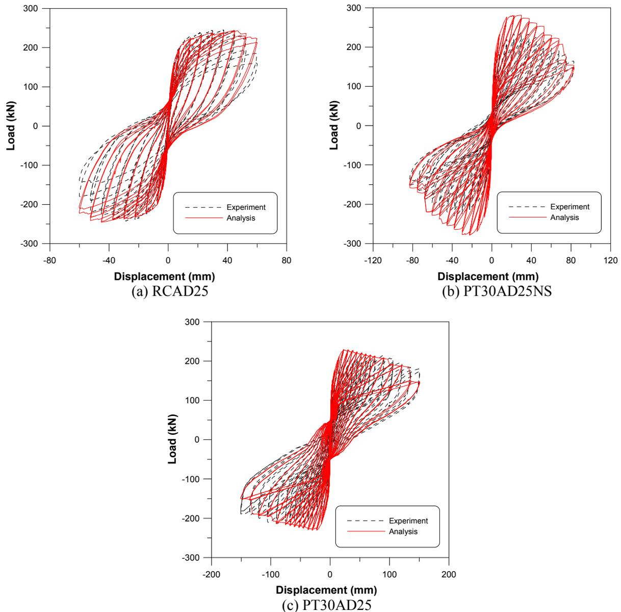
Figure 6 Comparison of results from the experimental results
