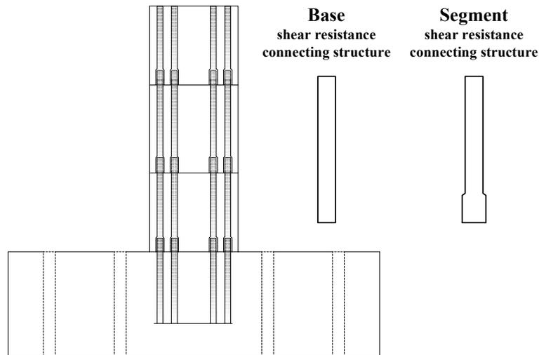
Figure 1 Proposed segmental bridge piers with shear resistance connecting structure
