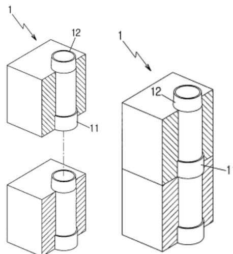
Figure 2 Design concepts of proposed shear resistance connecting structure
