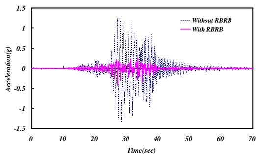
Figure 14 Absolute accelerations of structure with and without MC-RBRBs under three-directional Chi-Chi earthquake (X=0.3g, Y=0.128g, Z=0.095g)
