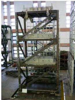
Figure 8 Three-story full scaled steel structure with MC-RBRBs
