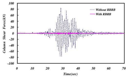
Figure 11 Column shear forces of structure with and without MC-RBRBs under three-directional Chi-Chi earthquake (X=0.3g, Y=0.128g, Z=0.095g)
