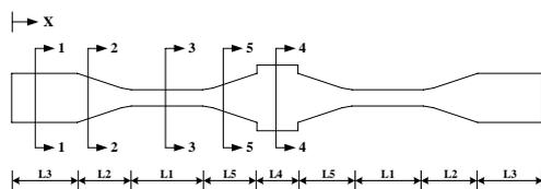
Figure 2 Sketch of the steel core of the multi-curved reinforced BRB
