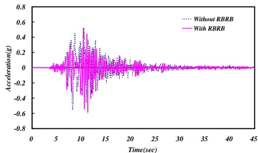
Figure 13 Absolute accelerations of structure with and without MC-RBRBs under three-directional Kobe earthquake (X=0.3g, Y=0.266g, Z=0.122g)
