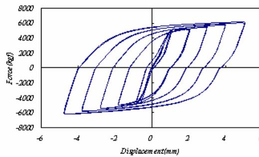
Figure 5 The hysteresis loops of the multi-curved reinforced BRB with a yield force of 4 tons
