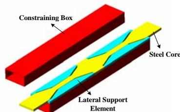
Figure 1 Sketch of multi-curved reinforced buckling restrained brace
