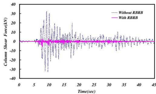
Figure 9 Column shear forces of structure with and without MC-RBRBs under three-directional El Centro earthquake (X=0.3g, Y=0.184g, Z=0.207g)
