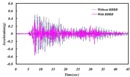
Figure 12 Absolute accelerations of structure with and without MC-RBRBs under three-directional El Centro earthquake (X=0.3g, Y=0.184g, Z=0.207g)
