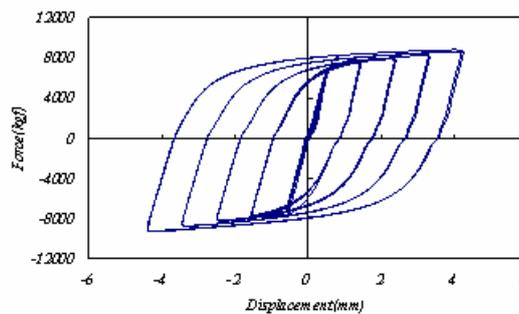
Figure 6 The hysteresis loops of the multi-curved reinforced BRB with a yield force of 6 tons
