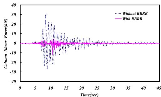
Figure 10 Column shear forces of structure with and without MC-RBRBs under three-directional Kobe earthquake (X=0.3g, Y=0.266g, Z=0.122g)
