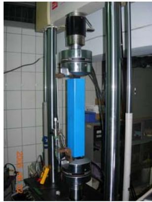
Figure 3 Test setup for the multi-curved reinforced BRB
