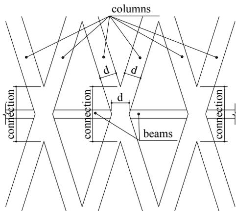
Figure 1 A typical connection in diagrid structures
