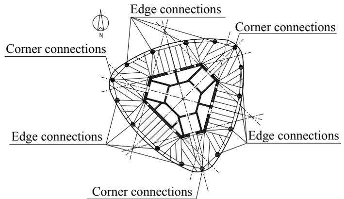
Figure 2 Corner and edge connections in the structure
