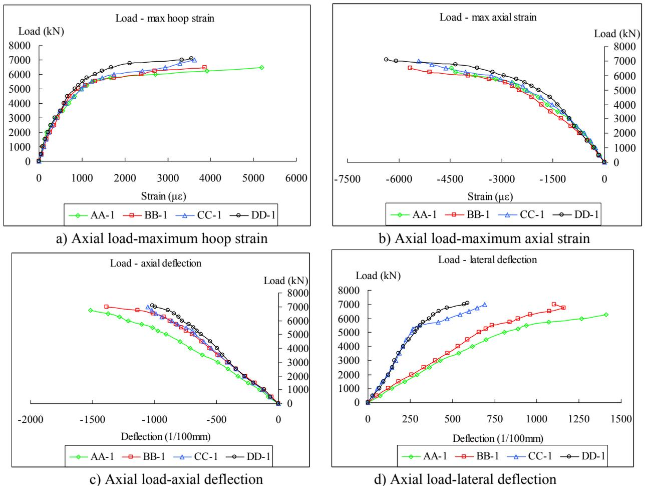
Figure 7 Load-steel strain and load-deflection curves
