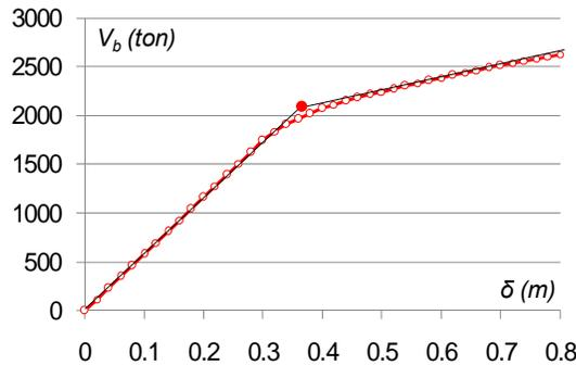
Figure 4. Capacity curve of braced building, nonlinear static analysis
