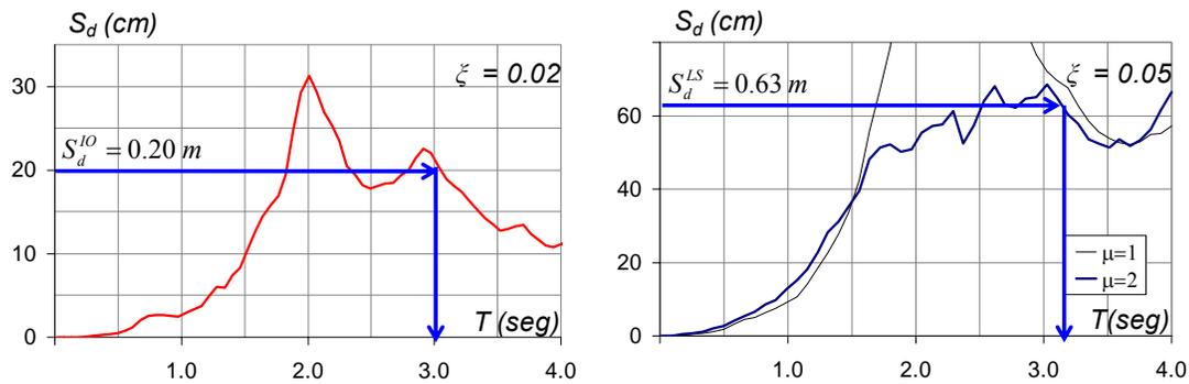
Figure 3. Design spectra for performance levels under consideration
