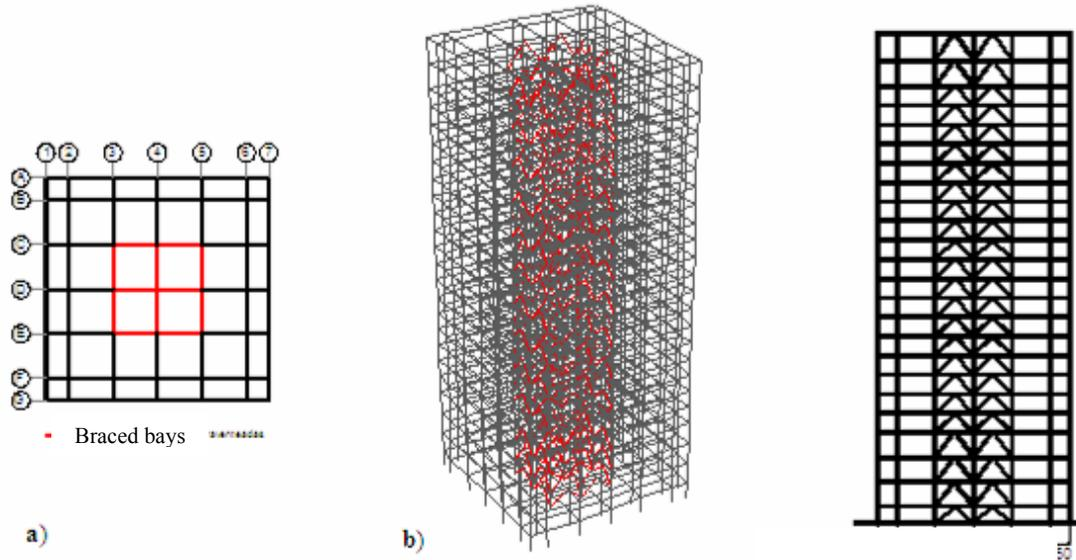
Figure 2. Geometry and structural layout of 24-story building. a) Plan, b) 3D model, c) Elevation
