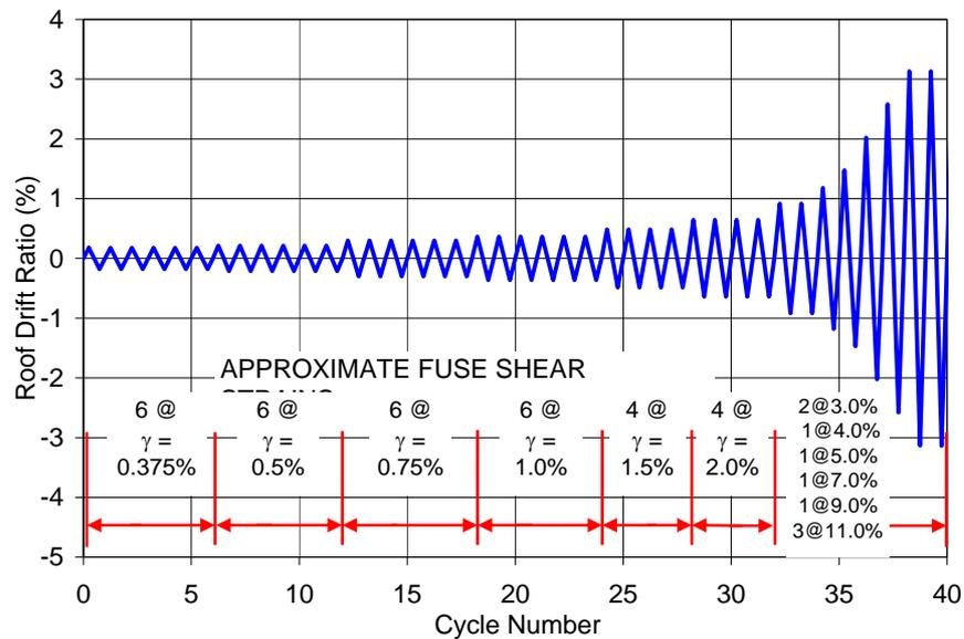
Figure 5 Displacement History Executed in Test A1
