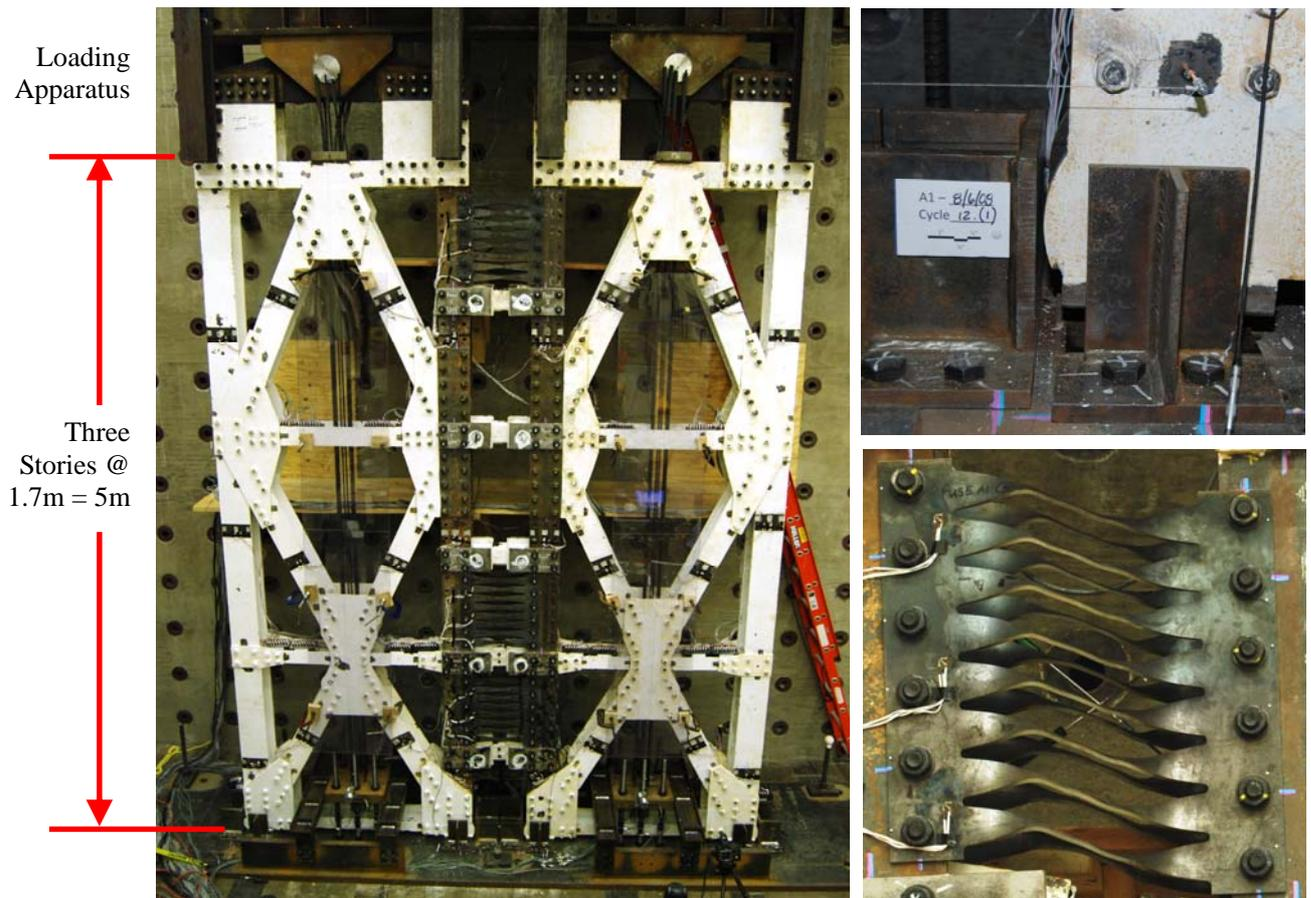
Figure 4 Half Scale Test Setup at UIUC (Left), Uplifted Base Connection (Top Right), Deformed Fuse (Bottom Right)
