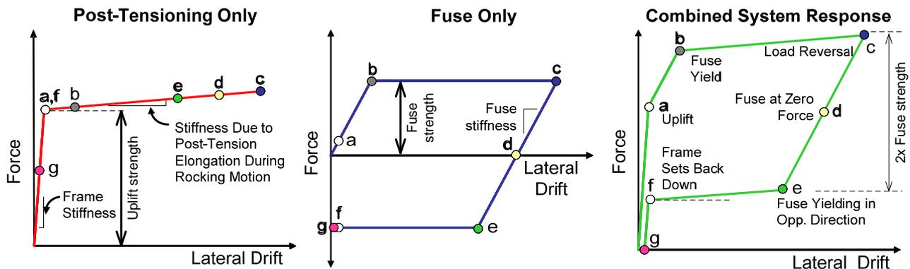
Figure 2 Schematic Depiction of the Controlled Rocking Hysteretic Response
