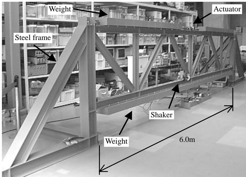
Figure 1 Large-scaled experimental model
