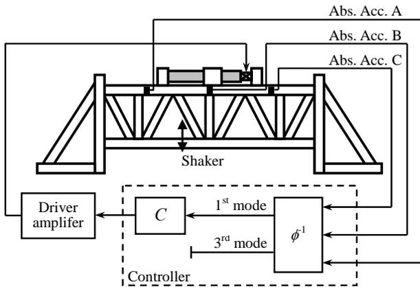
Figure 10 Control system for the experimental model
