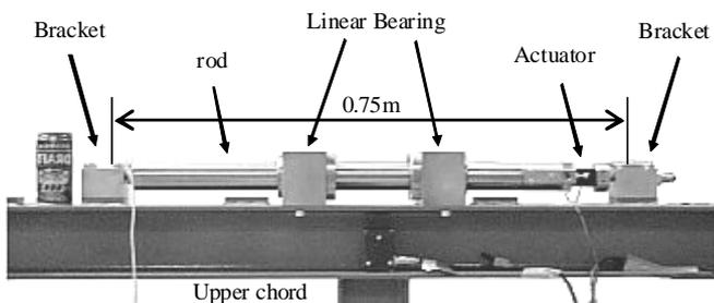
Figure 2 Installation of actuator on upper chord
