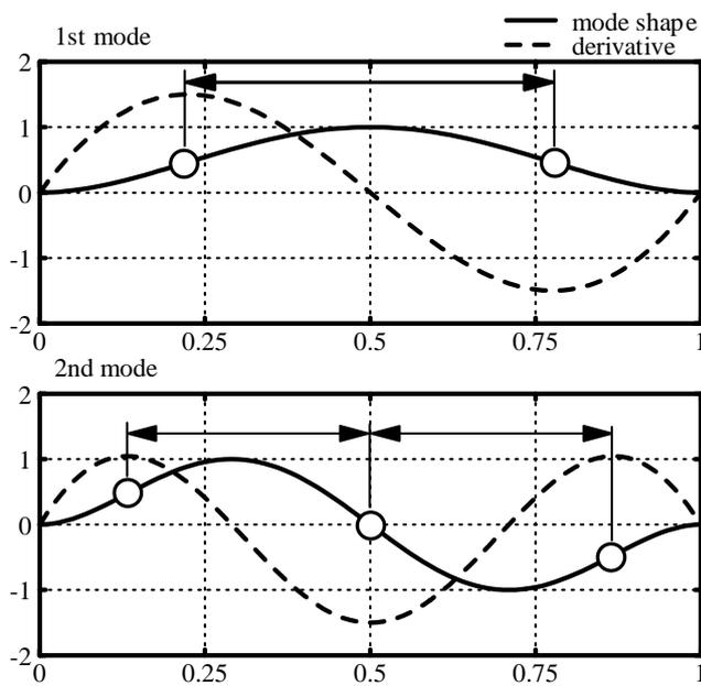
Figure 5 Mode shape functions and their derivative
