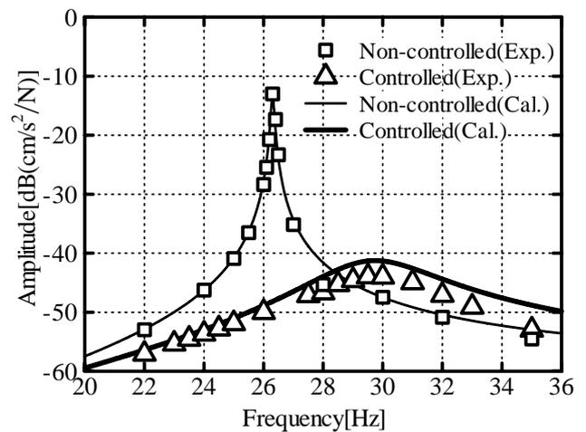
Figure 11 Vibration control performance
