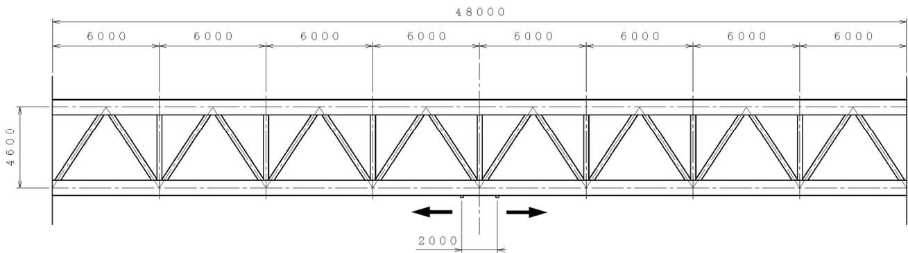
Figure 17 Supposed floor structure for the estimation of the proposed system
