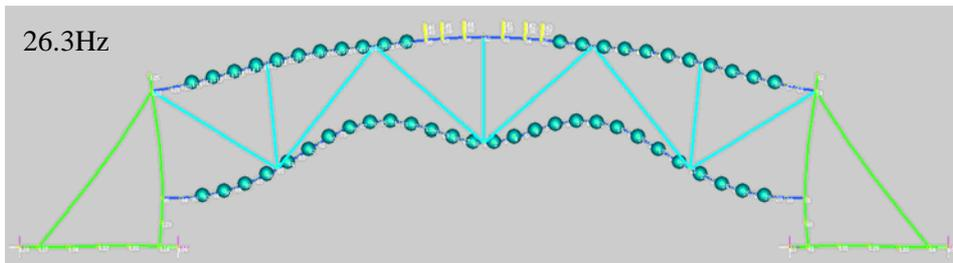
Figure 7 Modal analysis of FEM for the experimental model
