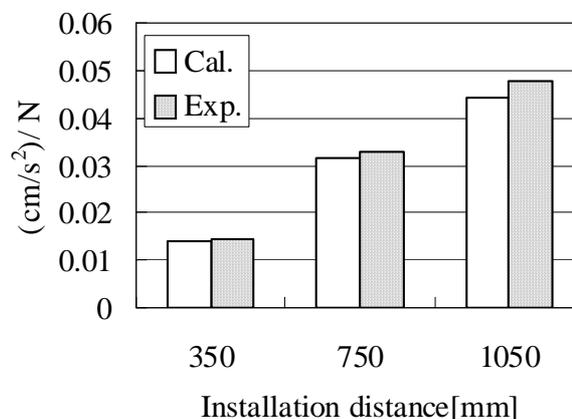
Figure 9 Results of the harmonic excitation by the actuator compared with the analysis
