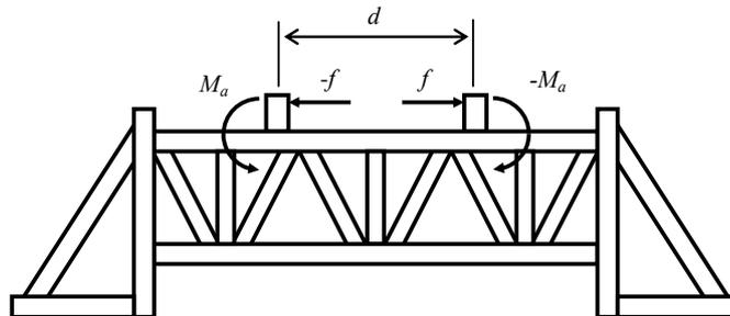
Figure 8 Outlines of the harmonic excitation test by the actuator
