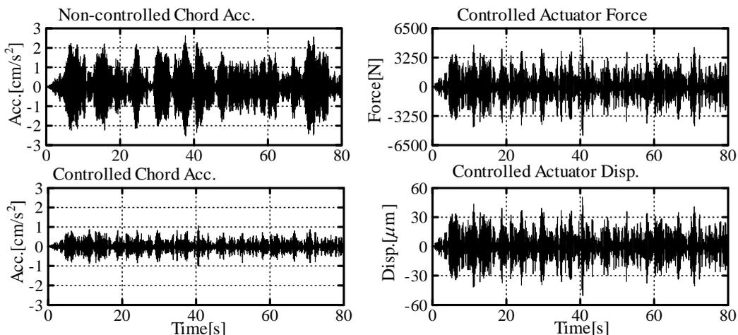
Figure 18 Estimated vibration control performance and actuator responses
