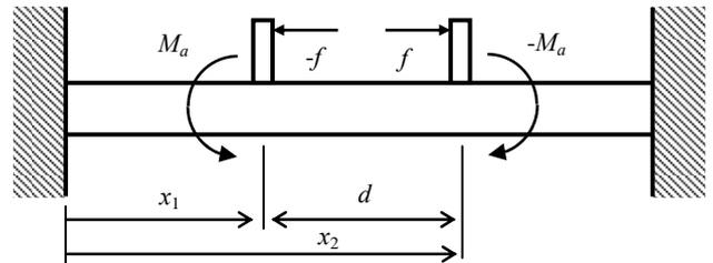
Figure 4 Analytical model of simple beam
