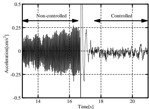
Figure 13 Time history when no excitation but ambient ground vibration was affected
