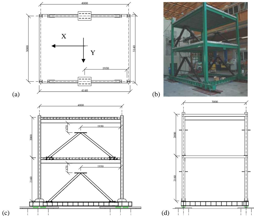
Figure 4 2:3 scaled steel frame built at the Structural Engineering Laboratory of the University of Basilicata in Potenza, Italy (Gattulli *et al*, 2007): a) plan view, b) 3D view, c) vertical plane XZ, d) vertical plane YZ.
