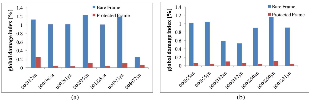
Figure 6: Global damage index for earthquakes compatible with Eurocode8: a) for type BCE soils in seismic zone 1, PGA=0.42g; b) for type A soil in seismic zone 1, PGA=0.35g.
