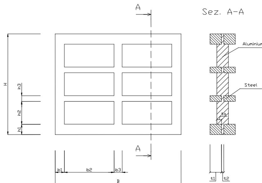
Figure 1 Geometrical parameters of the aluminium device.
