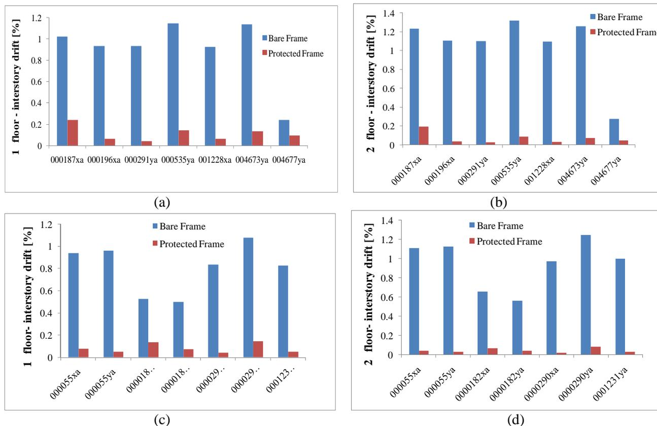
Figure 7 Maximum interstorey drift index: earthquakes compatible with Eurocode8 for type BCE soils in seismic zone 1, PGA=0.42g a) 1° floor and b) 2° floor; earthquakes compatible with Eurocode8 for type A soil in seismic zone 1, PGA=0.35g c) 1° floor and d) 2° floor.
