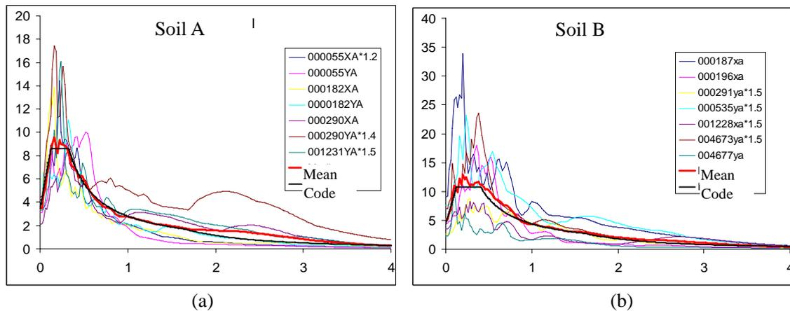
Figure 5 a) Response spectrum of considered natural earthquakes compatible with Eurocode8 for type A soil in seismic zone 1, PGA=0.35g; b) Response spectrum of considered natural earthquakes compatible with Eurocode8 for type BCE soils in seismic zone 1, PGA=0.42g (Ponzo *et al.* (2007))
