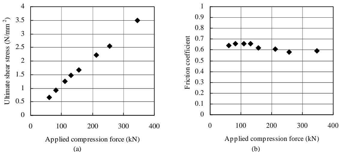
Figure 3.2 Ultimate shear stress and friction coefficient
