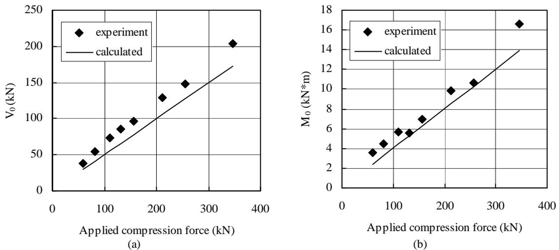
Figure 3.4 Relationship between applied compression force,  $V_0$  and  $M_0$
