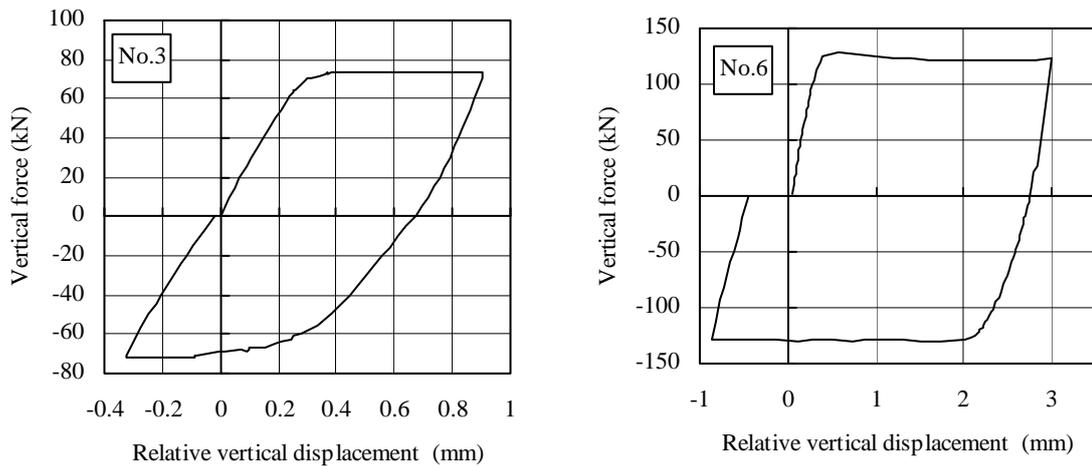
Figure 3.1 Relationship between relative displacement and vertical force (one connection)
