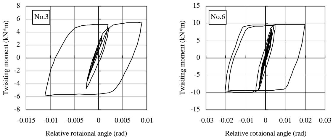
Figure 3.3 Relationship between relative rotational angle and twisting moment
