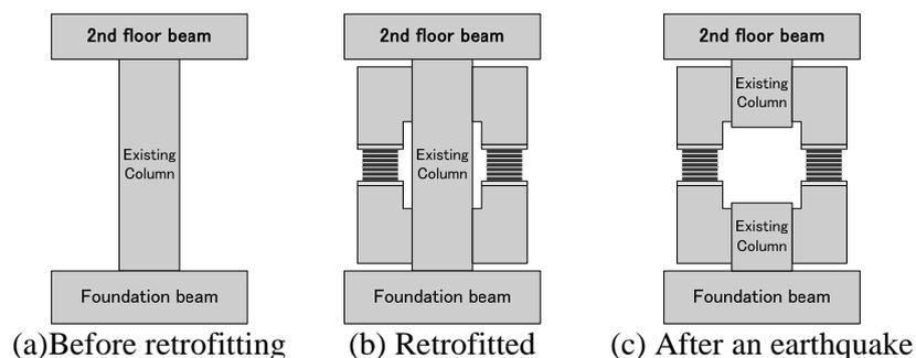
Figure 1.1 concept of the soft-landing base-isolation system
