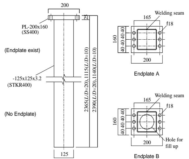
Figure 1 Specimen (mm)
