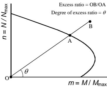
Figure 5 Definition of excess ratio
