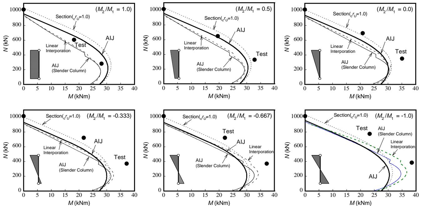
(b)  $L_h/D=10$  (Middle-length column),  $\sigma_B=27\text{N/mm}^2$
