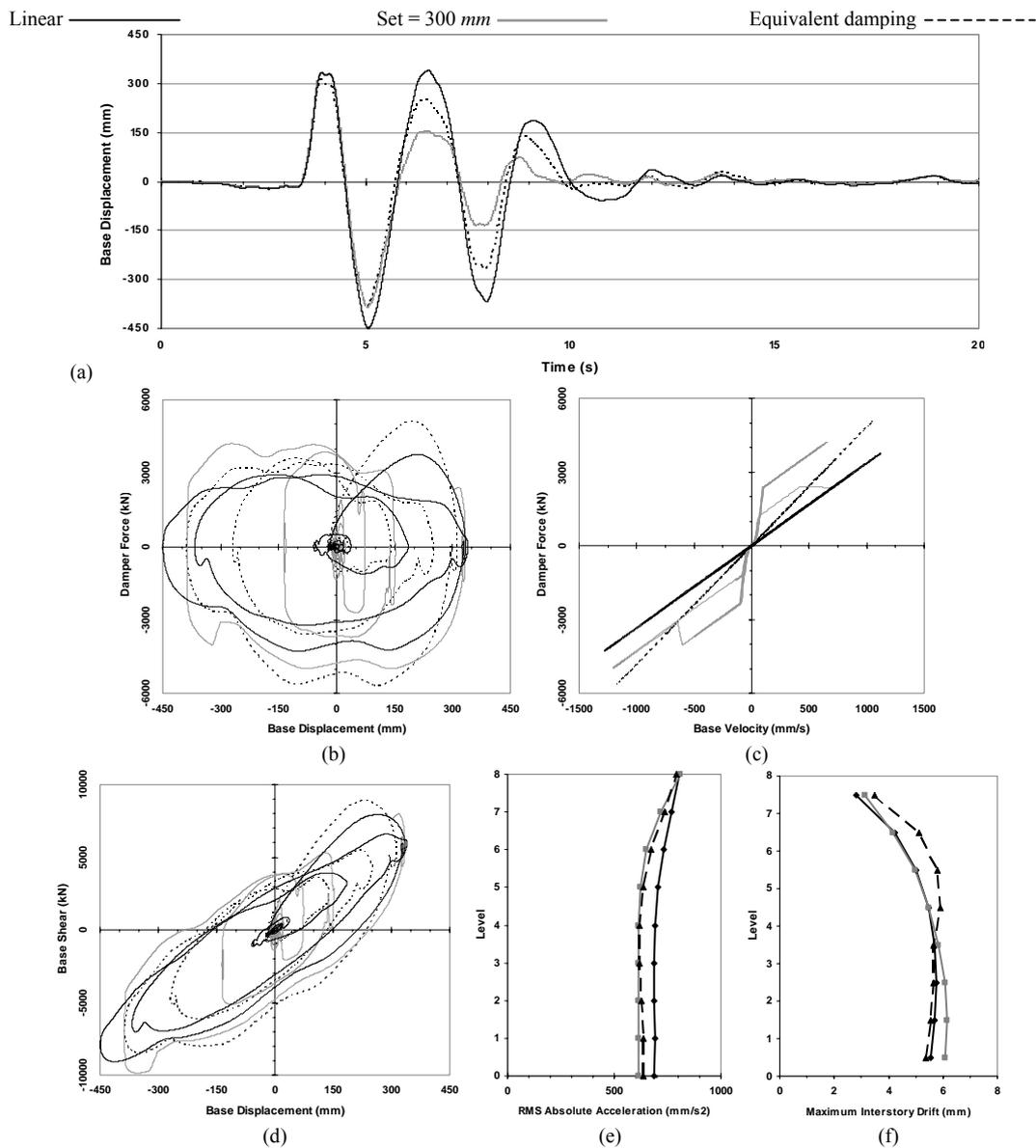
Figure 10. Comparison of response of 8-story base isolated system with VOD ( $F_V/w_{tot} = 6\%$ ) subjected to Sylmar earthquake when damper response is normal (set length > 449 mm) or nonlinear (set length = 300 mm) and equivalent linear damping: (a) Base displacement Time history; (b) Damper force vs. Base displacement; (c) Damper force vs. Base velocity; (d) Base shear vs. Base displacement; (e) RMS absolute acceleration distribution; and (f) Maximum interstorey drift distribution
