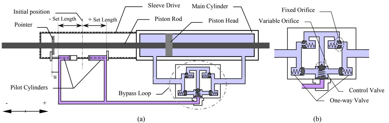
Figure 2. Variable Oil Damper: (a) Schematic diagram of VOD; and (b) Bypass loop detail
