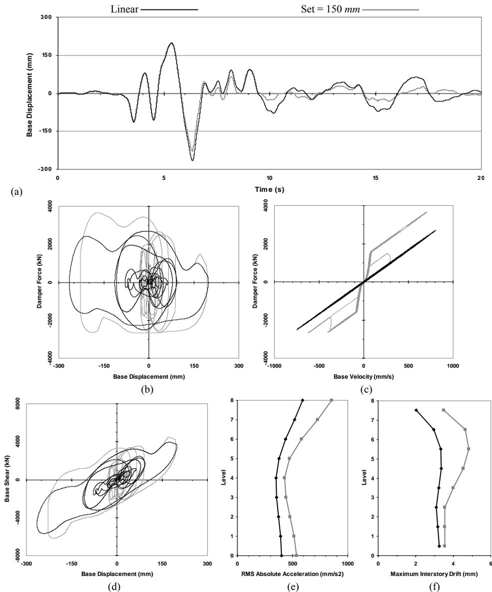
Figure 9. Comparison of analytical simulation results of 8-story base isolated system with VOD ( $F_d/w_{tot} = 4\%$ ) subjected to Kobe earthquake when damper response is normal (set length  $> 265$  mm) or nonlinear (set length = 150 mm): (a) Base displacement Time history; (b) Damper force vs. Base displacement; (c) Damper force vs. Base velocity; (d) Base shear vs. Base displacement; (e) RMS absolute acceleration distribution; and (f) Maximum interstory drift distribution
