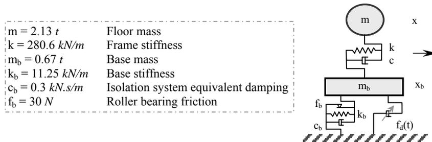
Figure 6. Schematic diagram of simulation model
