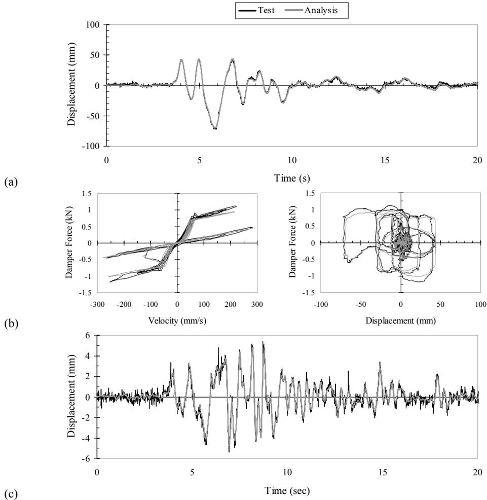
Figure 7. Comparison of experimental and analytical simulation results of 2-DOF system subjected to scaled Kobe earthquake when set = 45 mm: (a) Base displacement time history; (b) Damper force vs. Velocity and Displacement; and (c) Relative displacement of floor respect to base time history.
