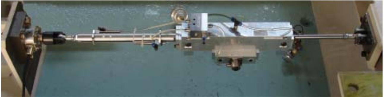
Figure 1. Photograph of variable oil damper (VOD)
