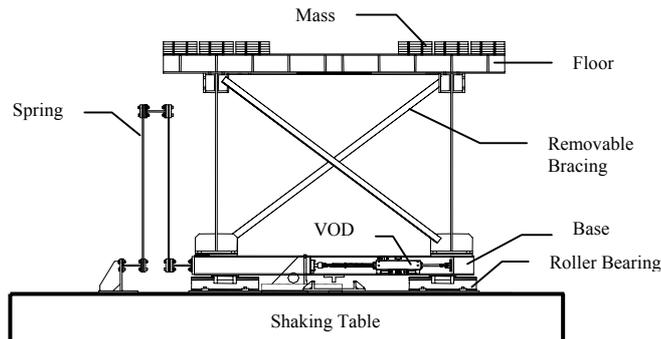
Figure 5. Details of model structure mounted on isolated base
