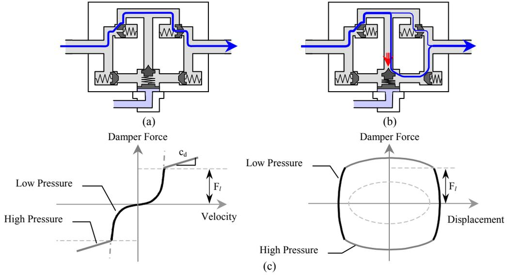
Figure 4. VOD behavior in nonlinear stage: (a) Bypass loop detail in low pressure; (b) Bypass loop detail in high pressure; and (c) Damper Force vs. Velocity and Displacement
