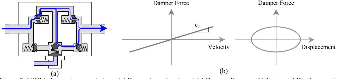
Figure 3. VOD behavior in normal stage: (a) Bypass loop detail; and (b) Damper Force vs. Velocity and Displacement
