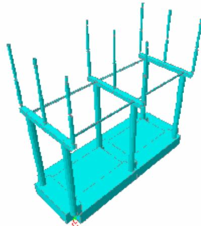
Figure 4.2 Model of isolated disconnector
