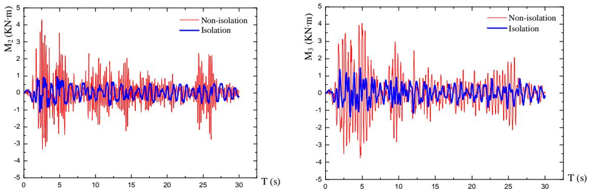
Figure 4.6 Time-history curves of bending moment under the wave of El-centro ( $620\text{cm/s}^2$ )
