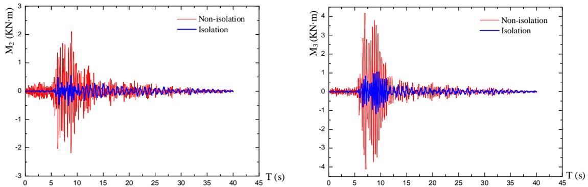
Figure 4.7 Time-history curves of bending moment under the wave of Taft (0.4g)
