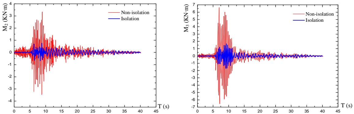
Figure 4.8 Time-history curves of bending moment under the wave of Tafts (620cm/s<sup>2</sup>)
