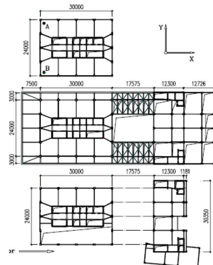
Figure 2 Typical plan layouts of SHIDC
