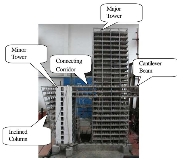
Figure 1 Structural elevation of SHIDC model
