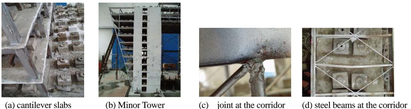
Figure 3 Failure pattern of SHIDC model
