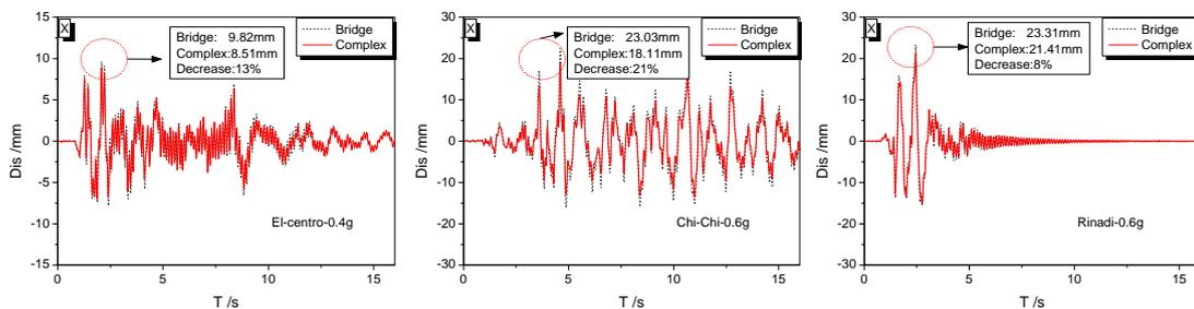
Figure 10 Comparison of the maximum displacement response between complex structure and bridge
