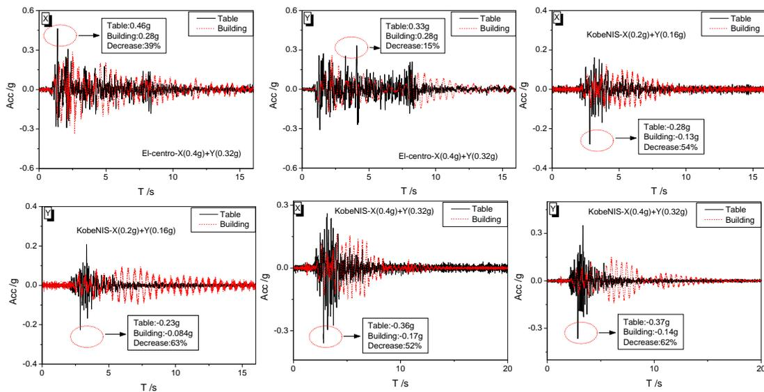
Figure 6 Comparison of the maximum acceleration response between building and table
