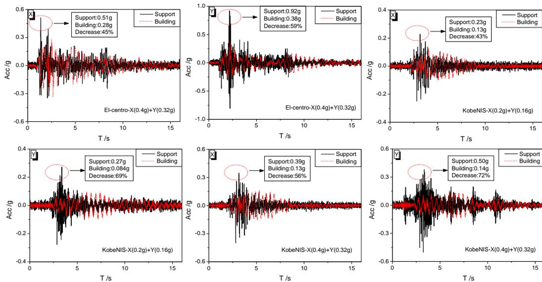
Figure 7 Comparison of the maximum acceleration response between building and support
