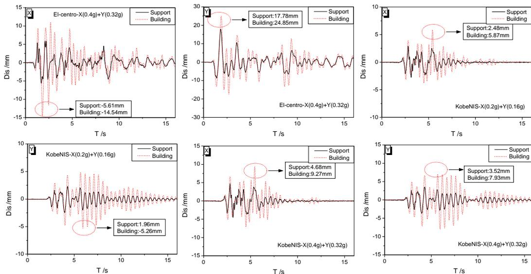
Figure 8 Comparison of the maximum displacement response between building and support
