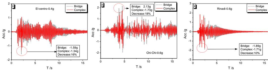
Figure 9 Comparison of the maximum acceleration response between complex structure and bridge
