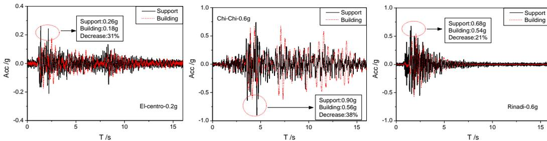
Figure 4 Comparison of the maximum acceleration response between building and support
