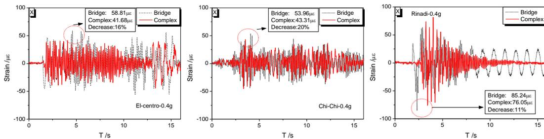
Figure 11 Comparison of the maximum strain-response between complex structure and bridge
