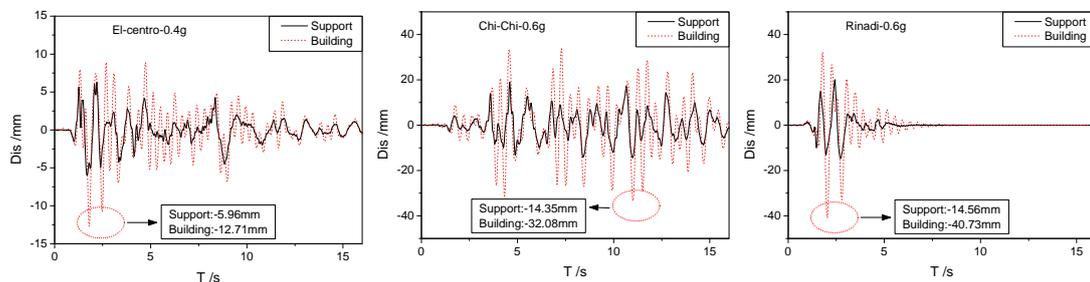
Figure 5 Comparison of the maximum displacement response between building and support
