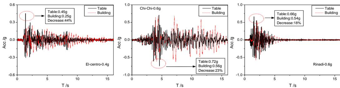
Figure 3 Comparison of the maximum acceleration response between building and table
