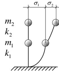
Figure 2 Analysis model of the complex structure
