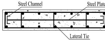
Figure 1 Schematic diagram for cross section
