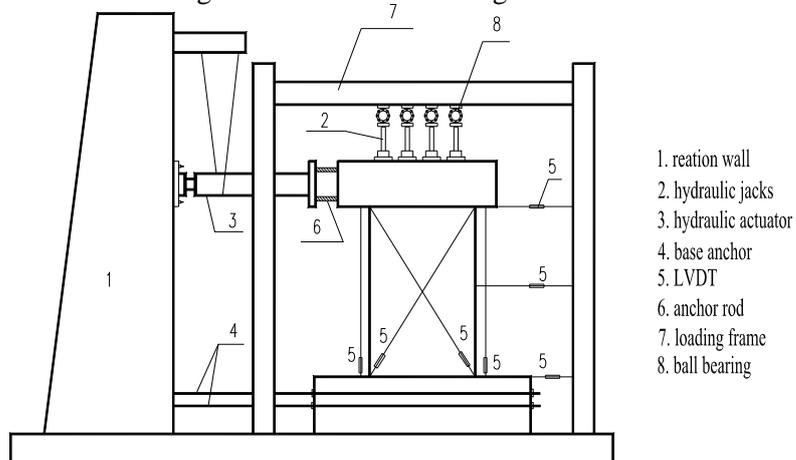
Figure 4 Test setup and instrumentation
