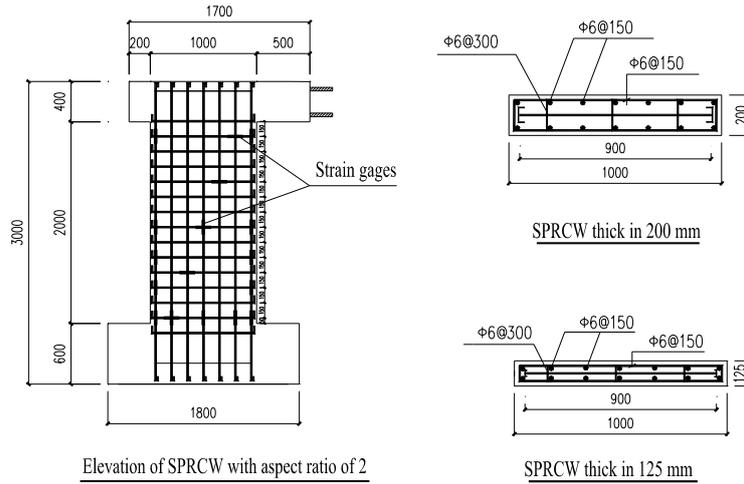
Figure 2 Diagram for reinforcement design
