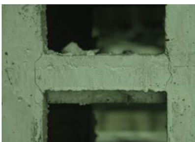
Figure 3 Cracks in coupling beam
