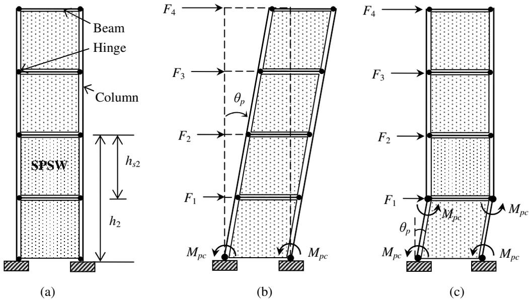
Figure 1 (a) Schematic of the SPSW system; (b) Selected yield mechanism; (c) Soft ground story [7]
