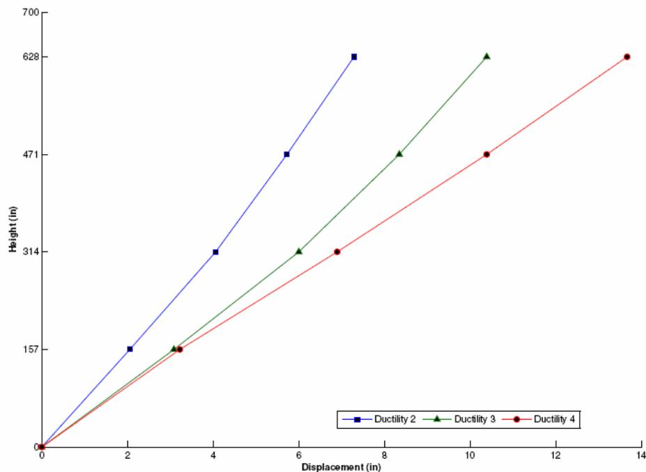
Figure 3 Displacement profiles at peak roof displacement for Designs I, II and III (1 in = 0.0254 m)
