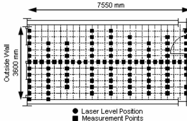
Figure 4 Plan view of the occupied office space and the measurement points
