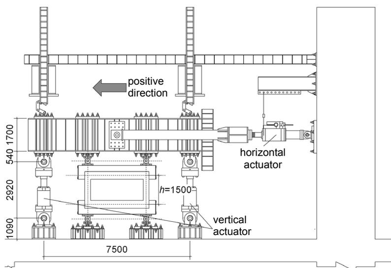
Figure 3 Dynamic loading apparatus
