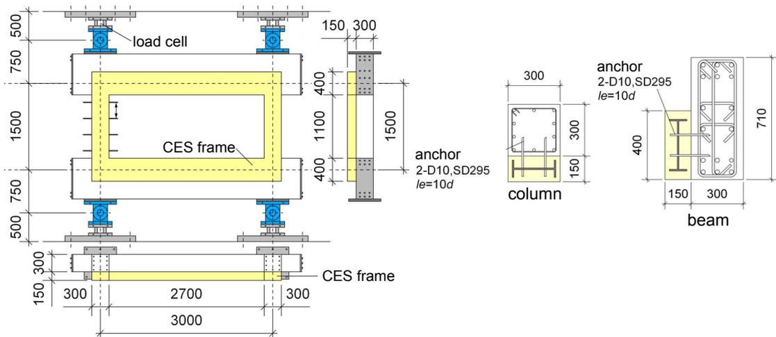
Figure 2 Test specimen
