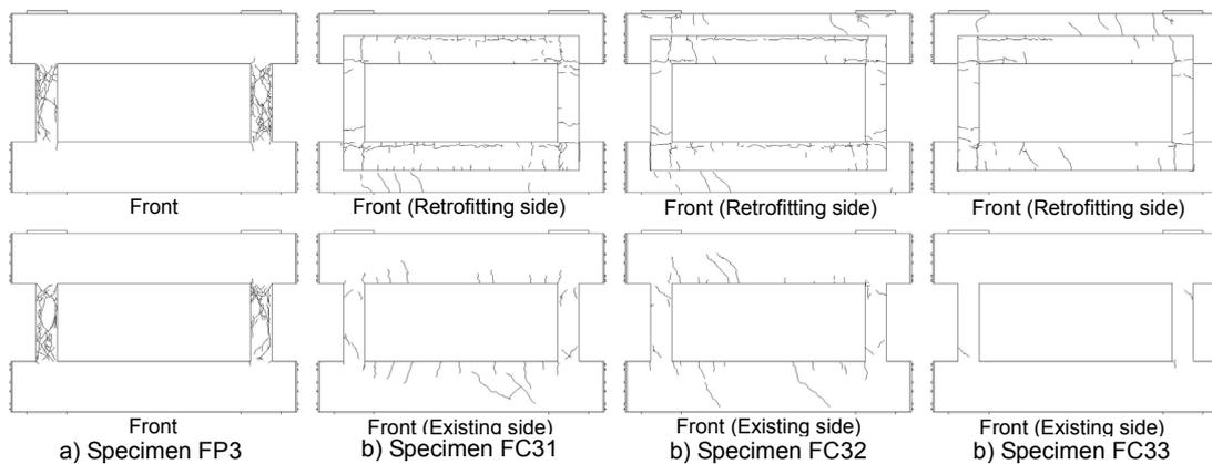
Figure 4 Crack conditions ( $R=0.01$  radians)
