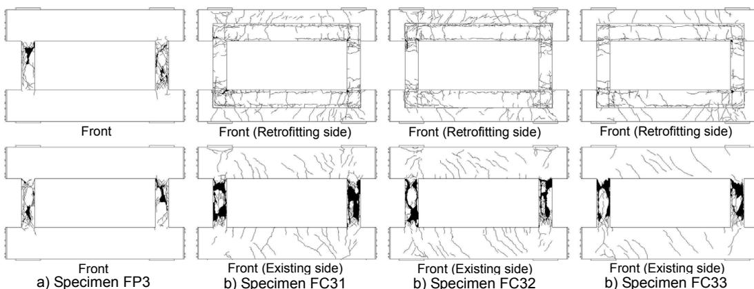
Figure 5 Final failure modes
