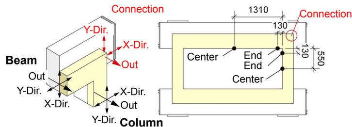
Figure 10 Definition in direction of each shearing and the measurement locations
