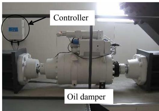
Figure 2 Installed semi-active oil damper
