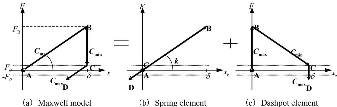
(a) Maxwell model (b) Spring element (c) Dashpot element
