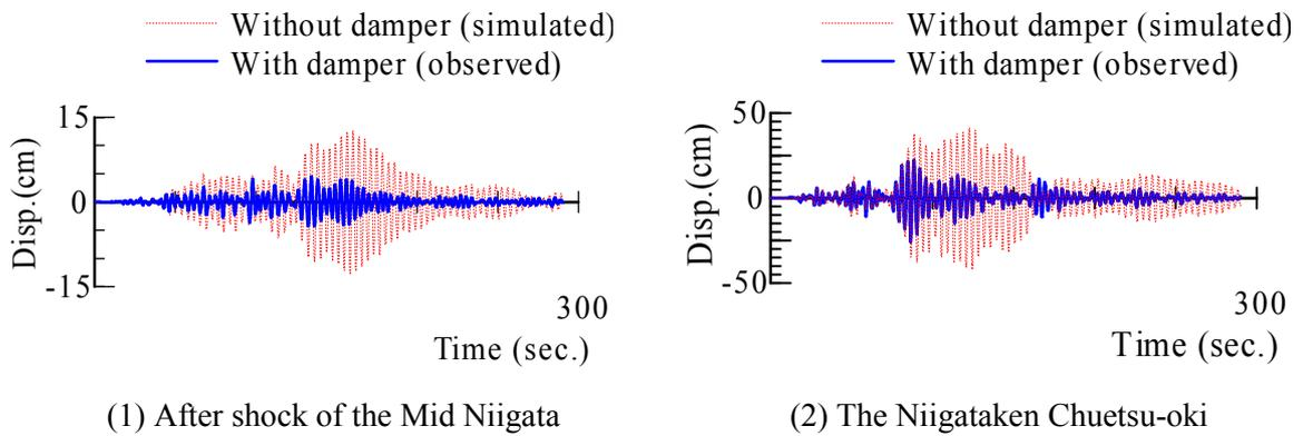
Figure 11 Control effect of semi-active oil damper
