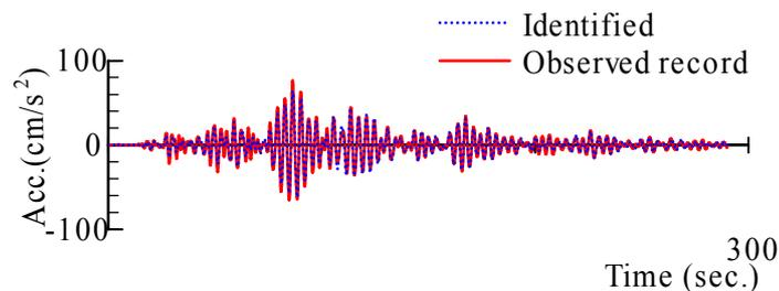
Figure 9 Transverse directional acceleration at roof floor
