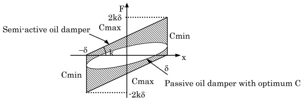
Figure 5 Force-displacement relation of dampers under harmonic excitation
