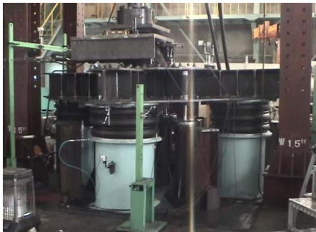
Figure 1.6 Photograph of 3D seismic isolation device
