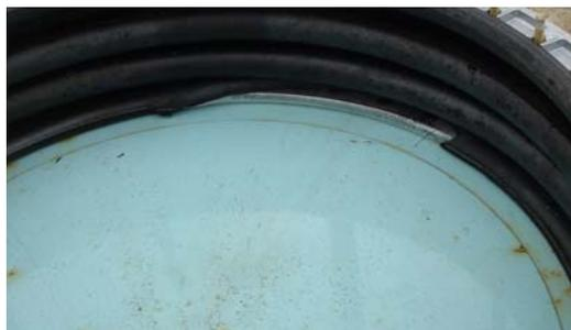
Figure 1.5 Breaking situation of rubber bellows (Device 1)
