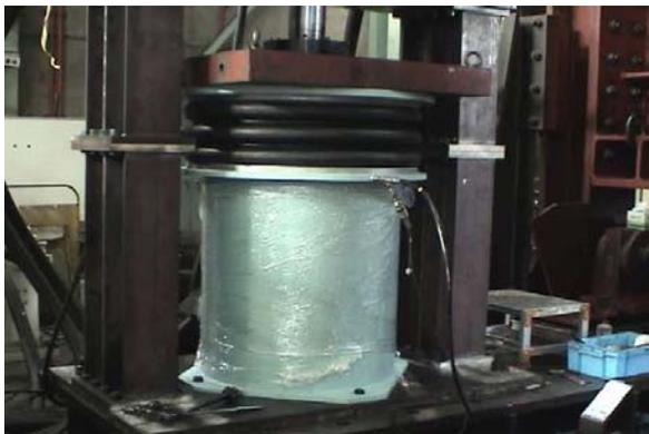
Figure 1.1 Photograph of Dynamic test of air spring
