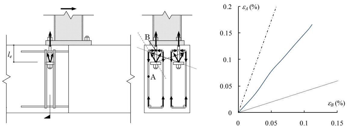
Figure 6 Strain distributions on transverse reinforcements around anchor bolt under tension
