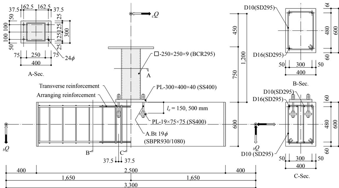
Figure 2 Details of test specimens
