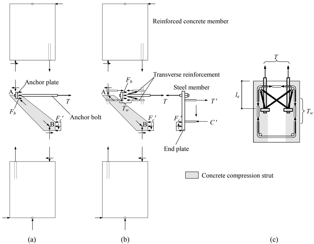
Figure 1 Stress transferring mechanism
