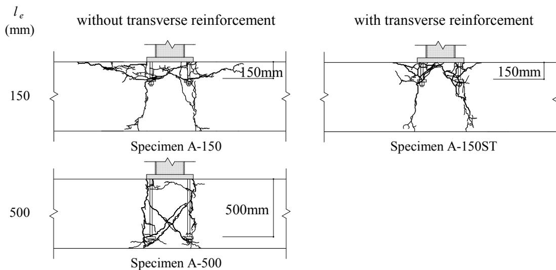
Figure 4 Crack Patterns
