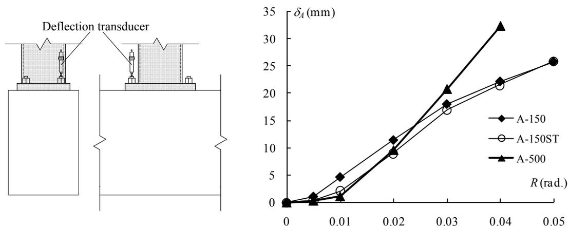
Figure 7 Relationships between pull-out displacement of anchor bolt under tension and drift angle
