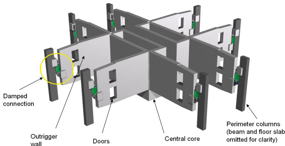
Figure 4 General arrangement of outrigger levels
