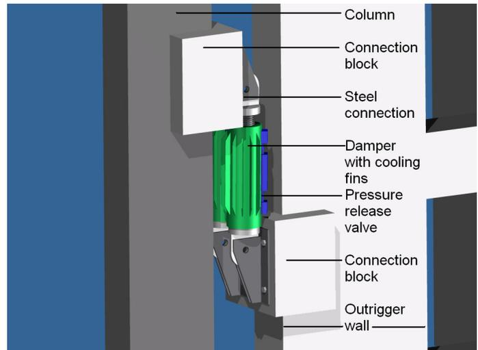
Figure 3 - Close up of damper connection detail
