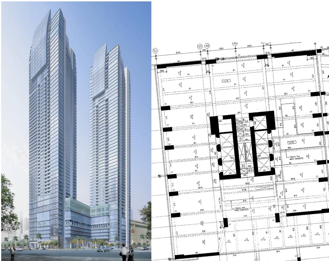
Figure 1 Architectural rendering of towers and structural plan of tower 2
