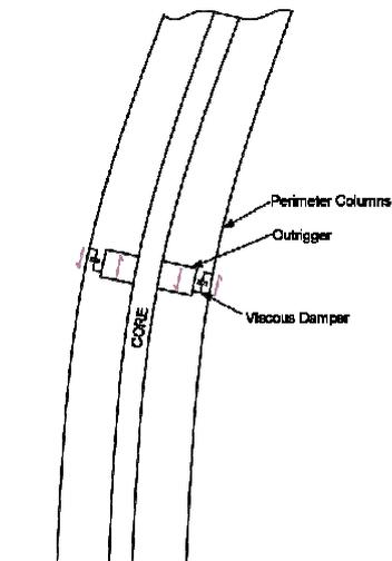
Figure 2 - Arup Damped Outrigger (patents pending)
