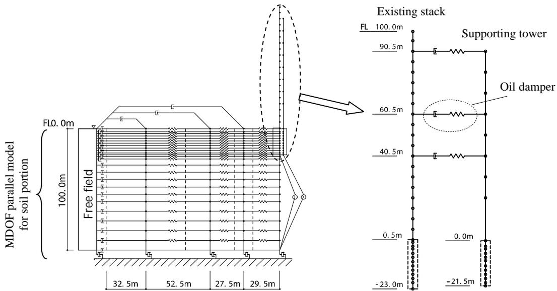
Figure 6 Vibration model for seismic response analysis
