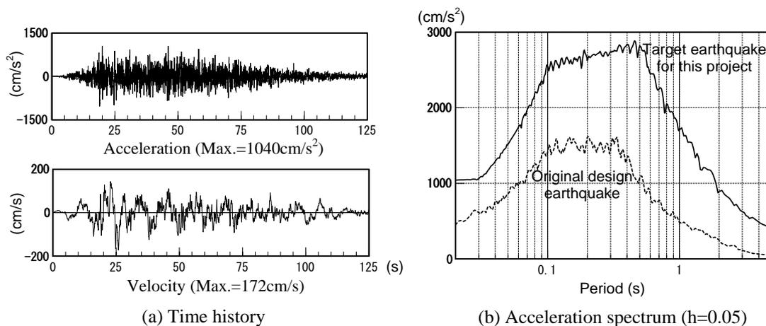
Figure 2 Target design earthquake
