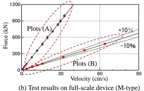
Figure 9 Force-velocity relation of oil damper
