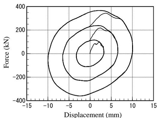
(a) Force-displacement relation for sinusoidal loading (2.0Hz)
