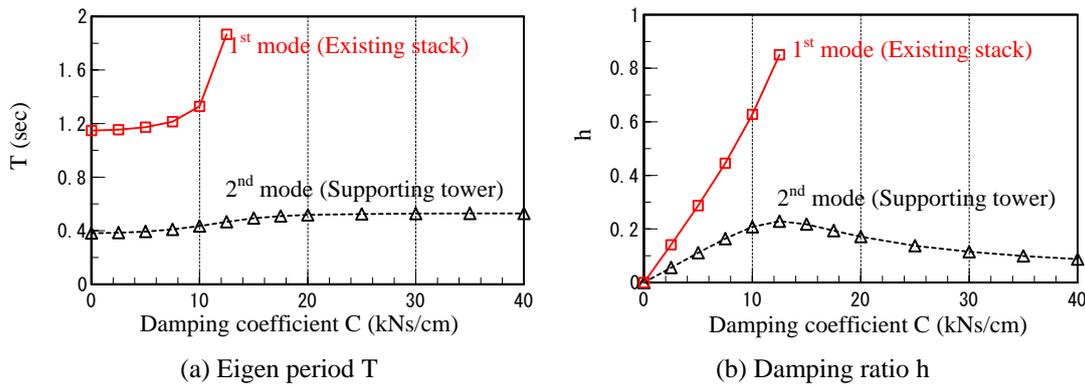
Figure 4 Complex eigen-values of fundamental modes
