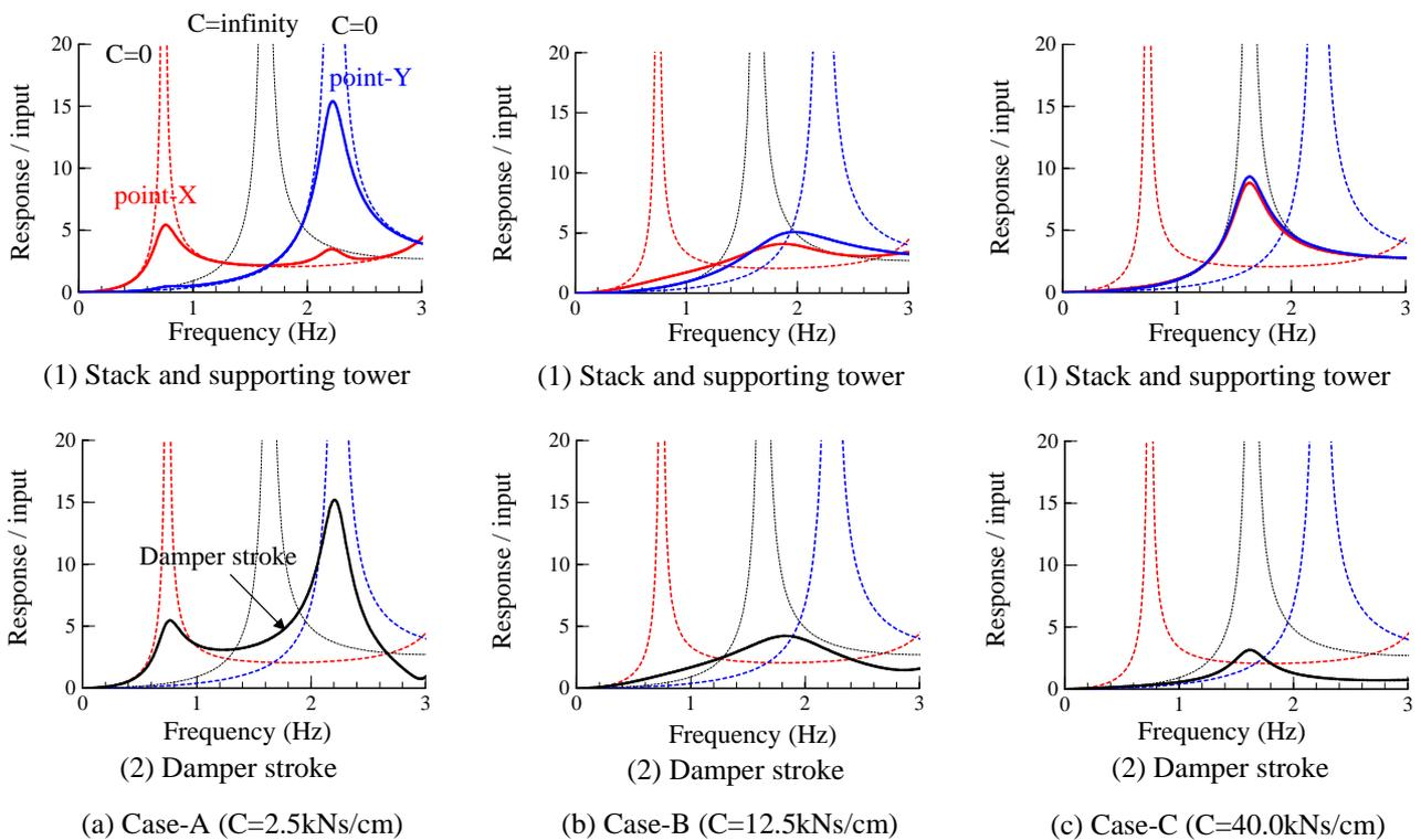
Figure 5 Resonance curves with various damper settings
