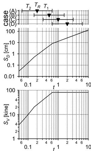
Figure 12 Modeled response spectrum
