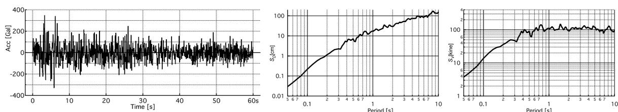
Figure 2 Time history and response spectrum ( $\xi = 2\%$ ) of input seismic wave
