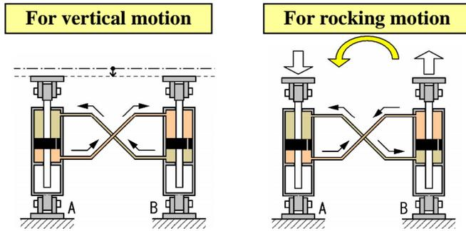
Figure 5 Mechanism of rocking suppression
