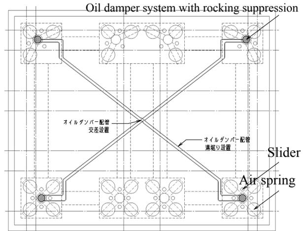
Figure 6 arrangement plan of Oil damper system with rocking suppression
