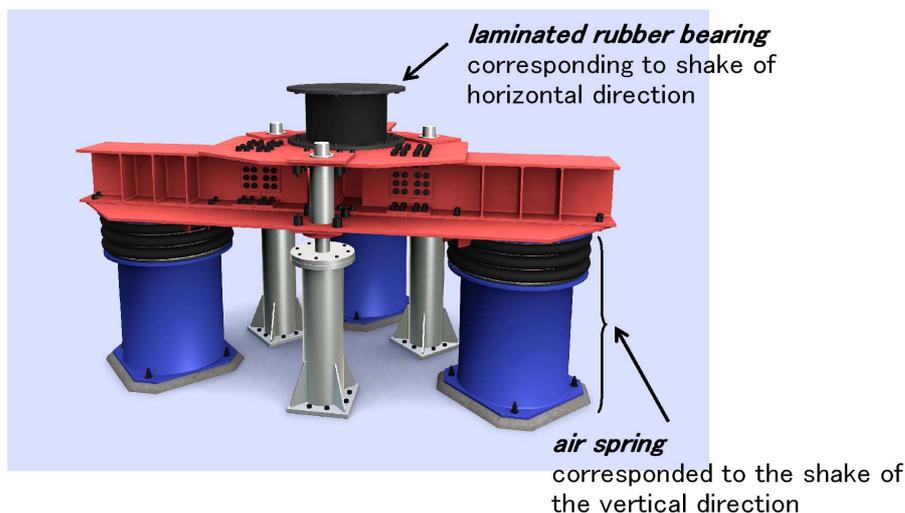
Figure 4 apparent of 3D seismic base isolation system
