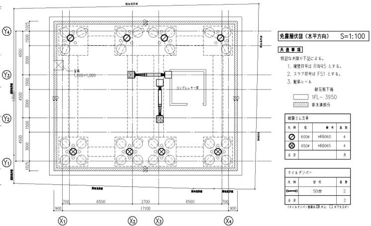
Figure 3 arrangement plan of seismic isolator's layer
