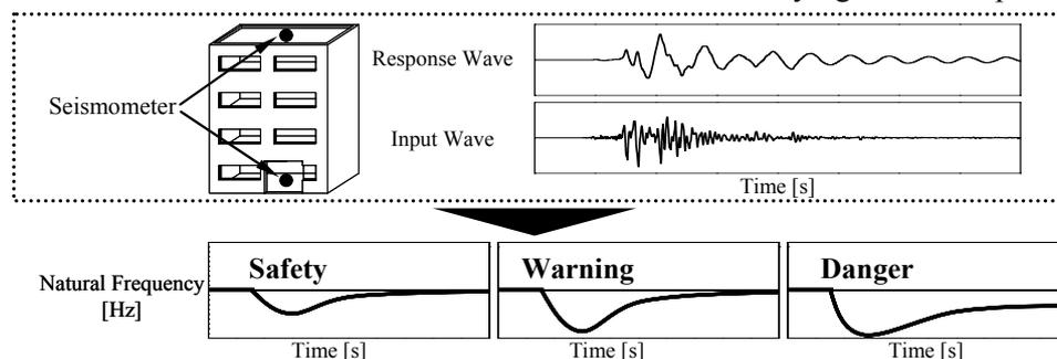
Figure 1 The application for structural health monitoring by using the transient change of natural frequency.
