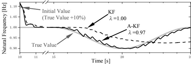
Figure 4 Comparison between the KF and the A-KF.
