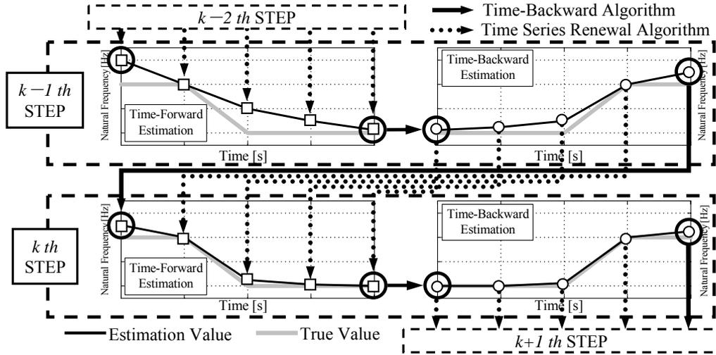
Figure 2 The flow of system identification by using the AFB-KF.
