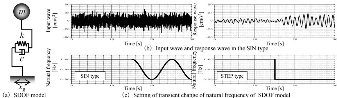
Figure 3 The SDOF model, input and response wave, and setting of natural frequency at numerical simulation.
