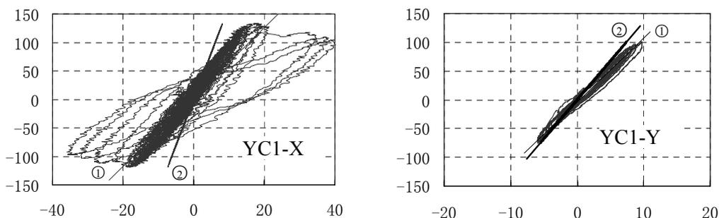
Figure 12 Rotation stiffness of bearing (kN: mm)
