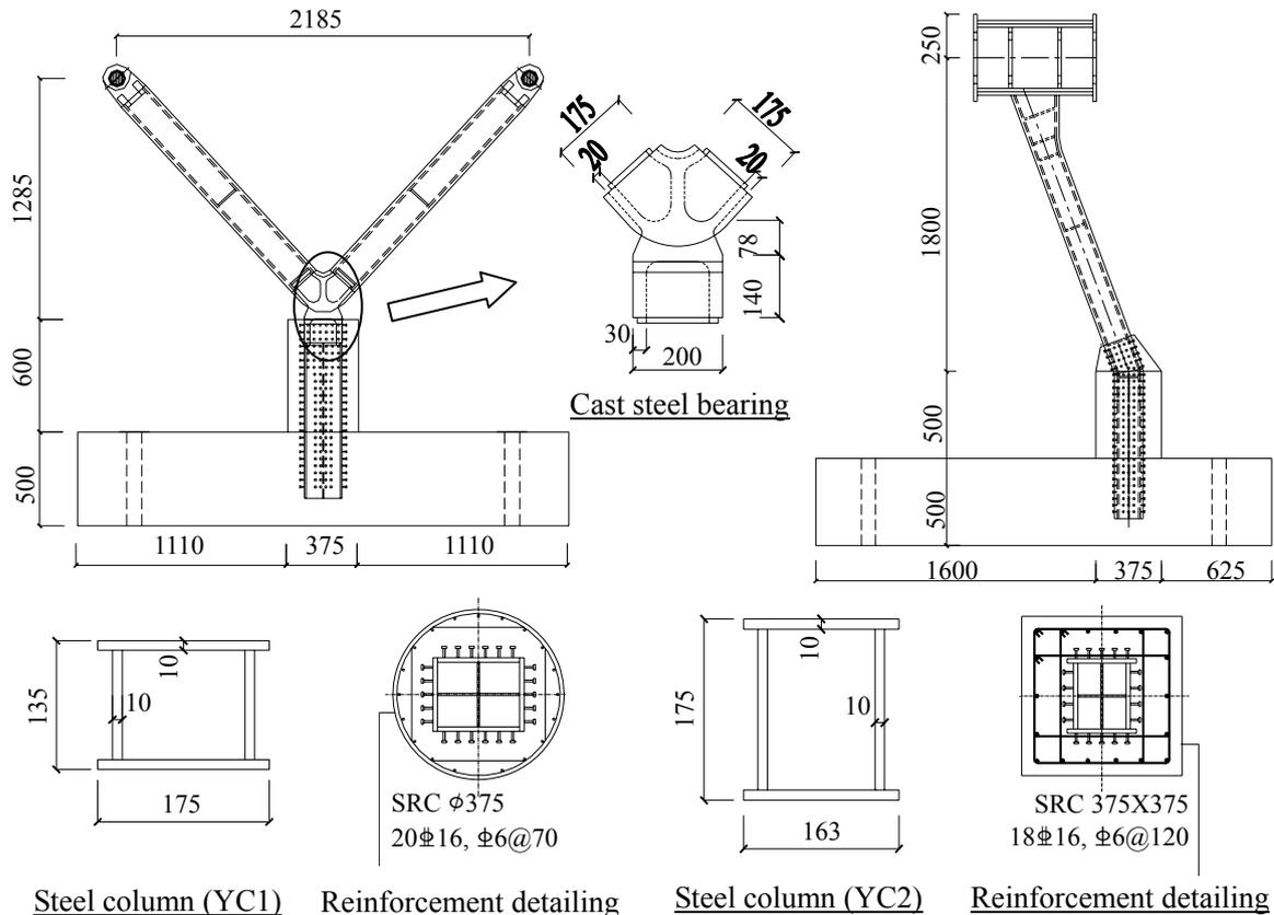
Figure 2 Detailing of specimen (mm)
