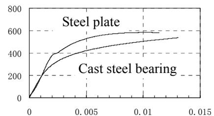
Figure 3 Property curves of steel (MPa: με)
