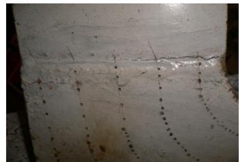
Figure 7 Cracks in HAZ of Steel
