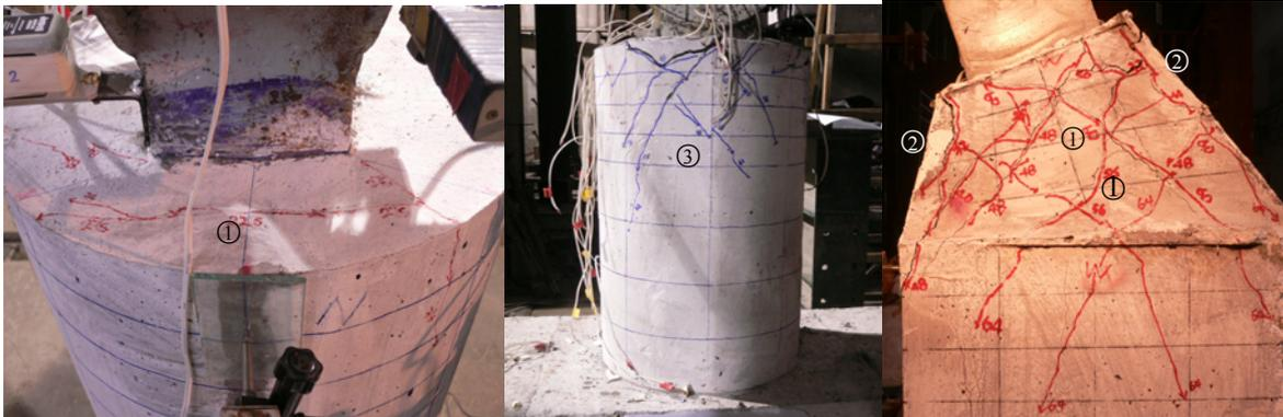
Figure 5 Cracks at the top of concrete column      Figure 6 Cracks on the body of concrete column
