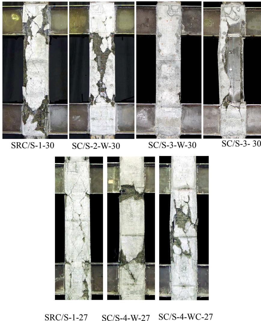
**Photo 1. The circumstances of the failures**
